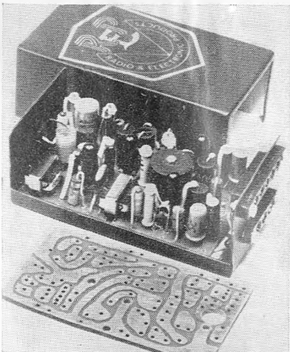
Above : The new R.E.P. reed bank and its component parts. Below : The "Twin-Triple" receiver and its P.C. board.
