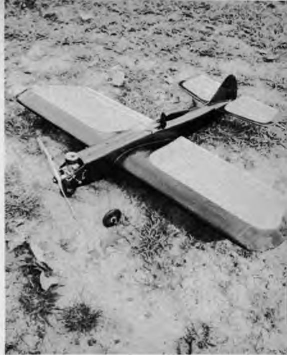
The tremendous wing area as well as the short tail moment arm make flying extremely easy.
