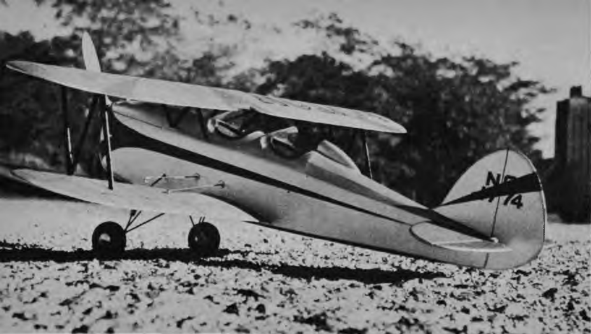
Note that the control-line leads extend about 4 inches from the side of the fuselage. The control-lines are first slipped through the guide on the wing struts and then hooked on to the leads.
