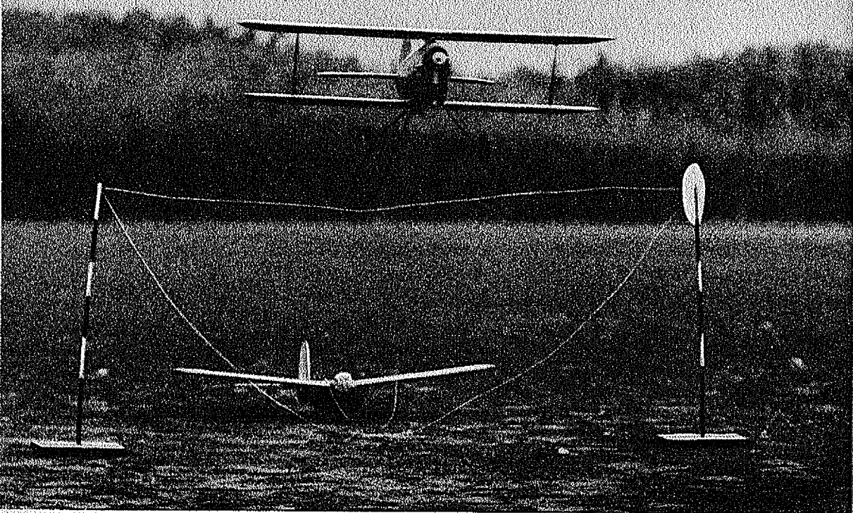
Action photo above taken at instant of snatch pick-up as tow plane swoops over glider station.
