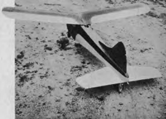
Plane ready for take-off. Tricycle landing gear gives model stability and protection.
