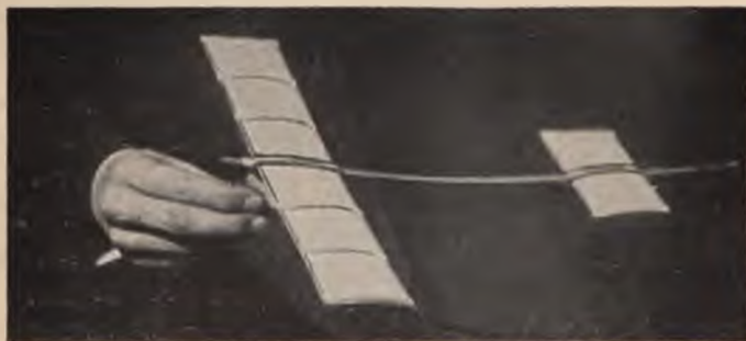
A covered-frame sling-shot glider
