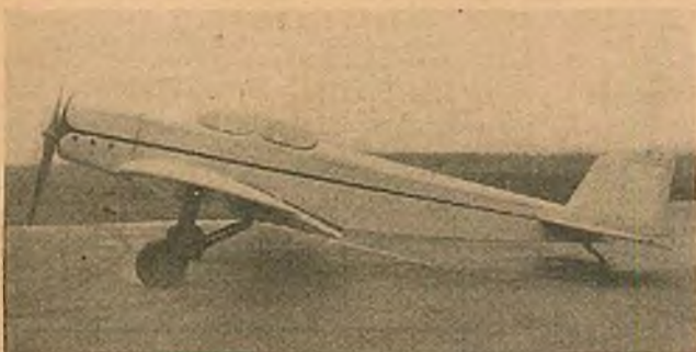
Keene Ace sportplane is powered by 82 h.p. Ford V-8 convertible auto engine.
