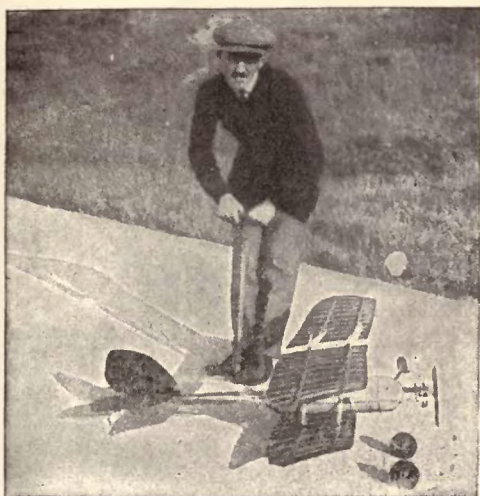
Frank Schober preparing his model for flight. Gauge to determine pressure of air may be seen in photograph
