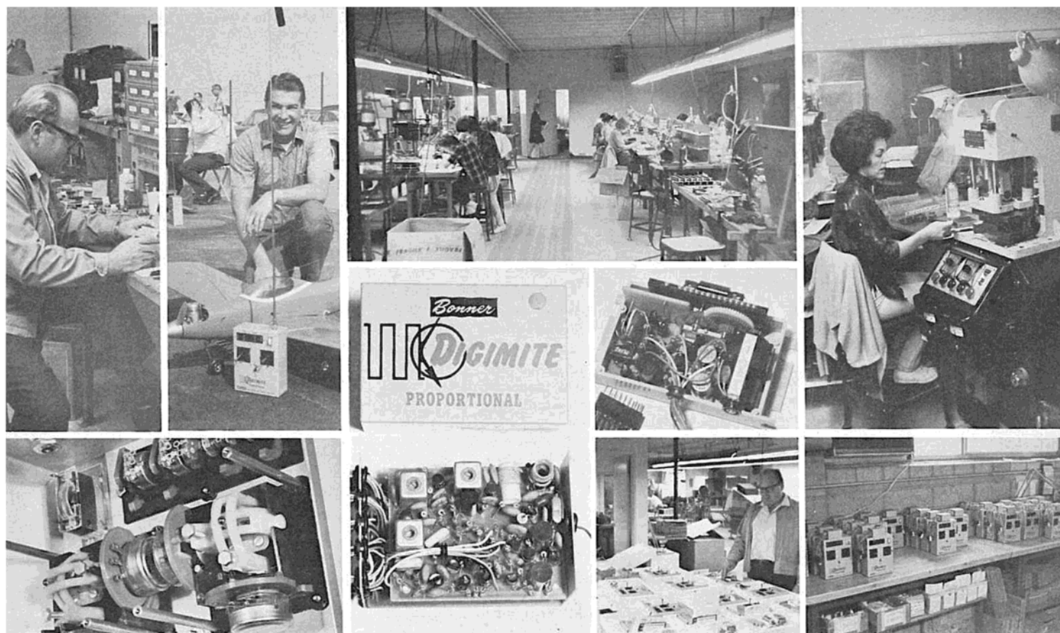
Top, L to R: Frank Justin checks out Digimite servo at Bonner Specialties; Chuck Waas and 'Candy' test ship; a portion of the assembly line at the Bonner plant; one of the steps in the Digimite production. Bottom, L to R: Unique Digimite stick assembly, photographed from inside rear of transmitter. Note mechanical trim feature; Digimite two-deck receiver; servo with half-shell removed — note ball bearings at top; Justin at final inspection; Digimite systems awaiting testing.
