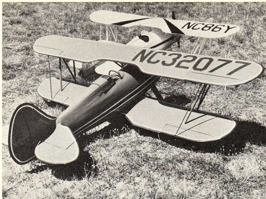
Frank Klotz's ZPF-7 was modified from the Dave Platt kit. Reshaped tail group and turtledeck, new sliding canopy and revised landing gear make this a distinctively different airplane.
