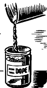
Silver powder, added to clear dope, gives "body" to fill pores of silk and nylon covering —
