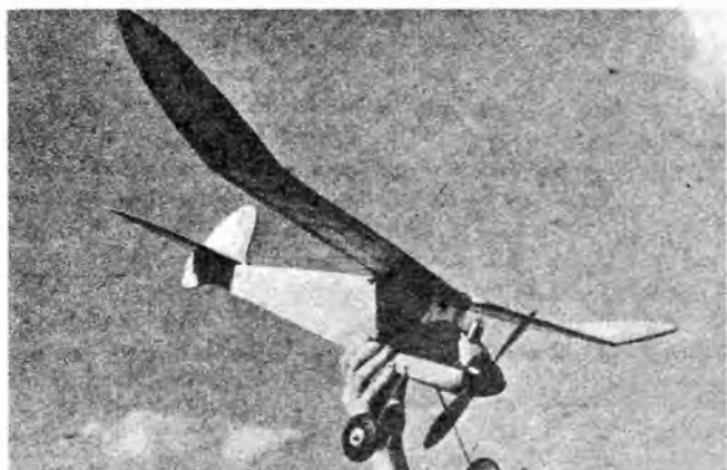
Mighty purty cabin free flighter built by R. A. Adams of London (who took these photos). Power supplied by Mills 1.3 cc diesel engine. Wing i.e. notched back above cabin. Clean construction.
