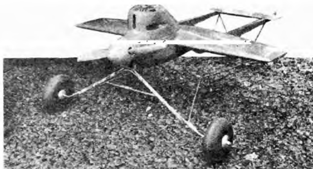
Unusual twin-boom speed job, powered by McCoy .60 engine designed and built by a Mr. Donovan (why won't Britishers give first names?), St. George's Heights MC. Pushrod runs atop port boom.
