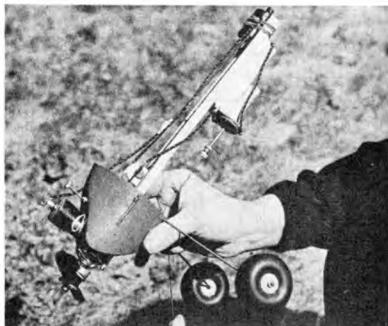
Timer is attached parallel to battery tray. Arm is pulled by cord running outside ship. Coil can be moved along tray for proper balance.
