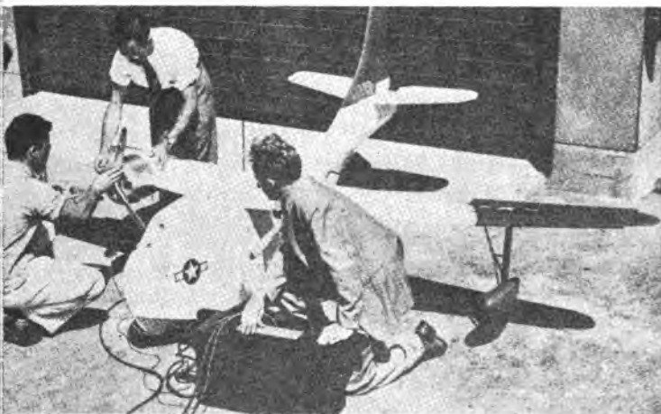
● Before flight of radio-controlled model, engineers test it thoroughly for proper engine and controls operation.
