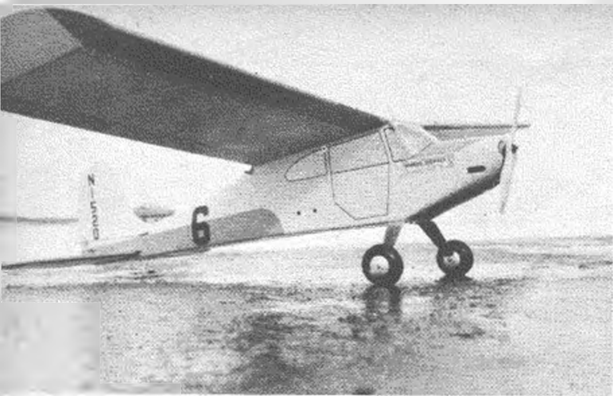
Aeronca-type Live Wire Champion, 56 in. span, 600 sq. in. area, for engines of .15 to .19 displacement. Has both elevator and rudder controls.
