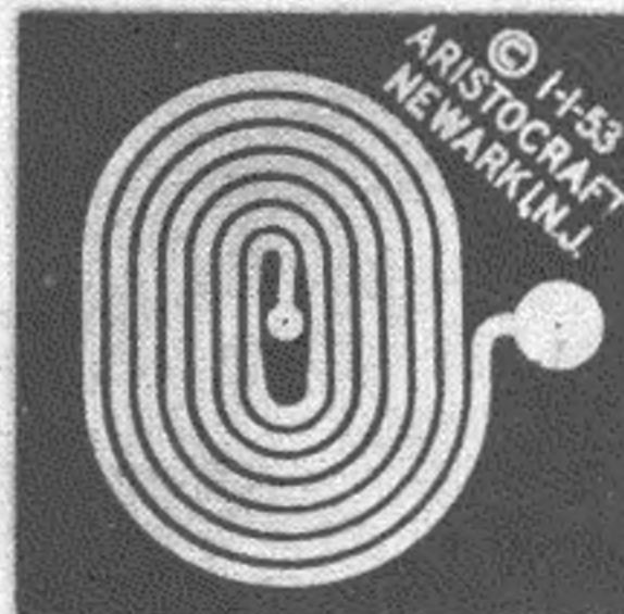
Examples of etched printed circuits. Although only .0014 of an in. thick, 1/64 in. wide copper strip will carry 3 amps, 1/8 in. up to 15 amps.
