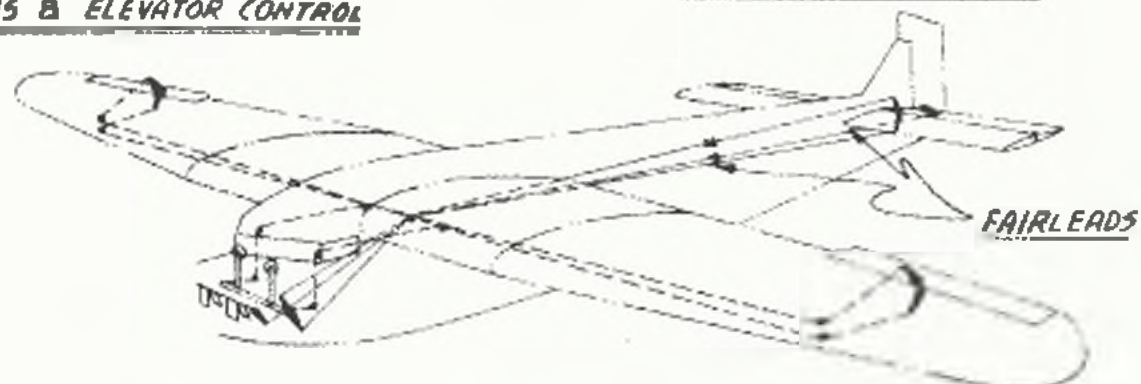
TYPICAL SURFACE CONTROL HOOK-UP
