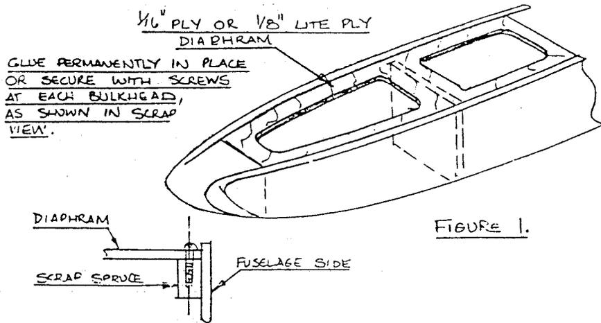
A considerable gain in fuselage rigidity can be made by adding a plywood diaphragm over the radio equipment bays, as shown in Figure 1. This can be glued in place after the servos are installed, or if you want to retain good access to the servos, the ply can be held in place with selftapping screws as shown in the detail figure. These should be at least six screws and they should be positioned midway between the fuselage formers. The diaphragm can
