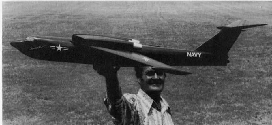
RON RAYMOND HOLDS ALOFT HIS BEAUTIFUL "SEAMASTER" POWER SCALE SLOPE SOARING DESIGN. WEIGHINF BUT OUNCES, THIS EXAMPLE OF FOAM AND PAPER IS RUGGED ENOUGH TO FLY THERMAL OR SLOPE WITH LIGHT-WEIGHT AIRBORNE FLIGHT PACKS. WEIGHS 7½ OUNCES! TAIL SURFACE A BIT SMALL AND WING AREA MAY BE ON THE LOW SIDE...SHOULD BE GOOD FLIER NONETHELESS.
