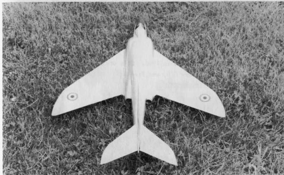
BEAUTIFUL TWIN-JET SWEEP-WING PSSS MACHINE SUITABLE FOR SLOPE OR THERMAL SOARING, DEPENDING ON THE SIZE AND AREA. CAN BE BUILT IN ONE-METER OR HALF-METER SIZES, BUT IS ALSO AMENABLE TO 1½-METER SIZE.
