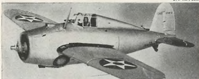
One of the most deadly of the navy's aerial weapons is the Grumman midwing fighter, XF4F-4, of exceptionally clean design. Note the machine-gun sight.
