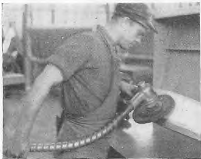
5. Grinding the blade to exact contour.
