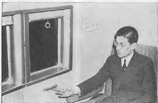
In each passenger compartment is an emergency door around one of the windows. Pulling of handle shown opens panel.
