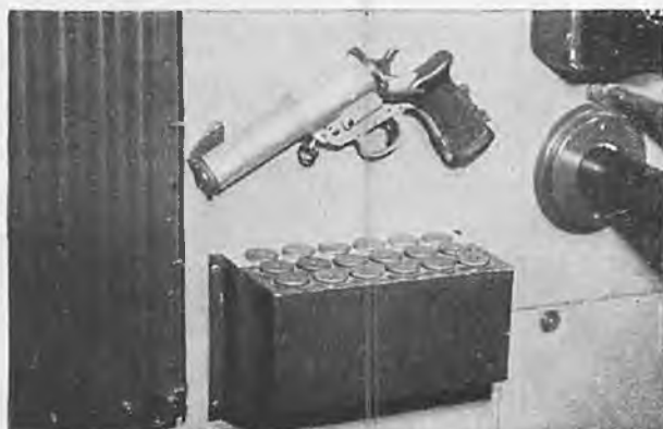
The often spoken of but seldom seen Very pistol for signaling with red, green and white flares in case of a landing at sea.
