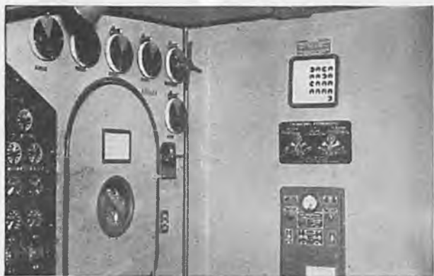
As a safety measure, these gauges indicate the exact amount of fuel in tanks. Engine fire extinguisher levers, center right.
