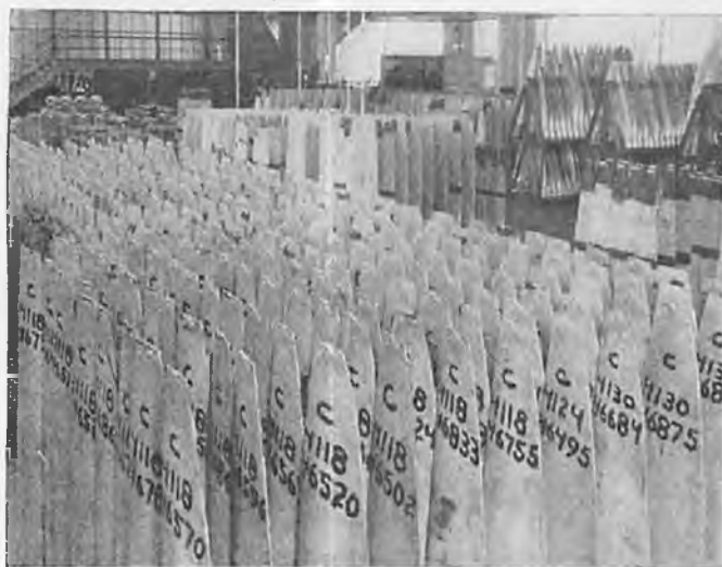
1. Blade forgings before machining.
