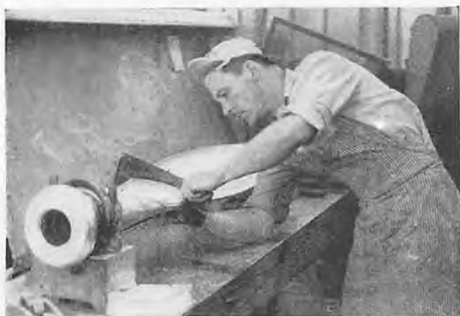
6. Template checking the grinding operation.
