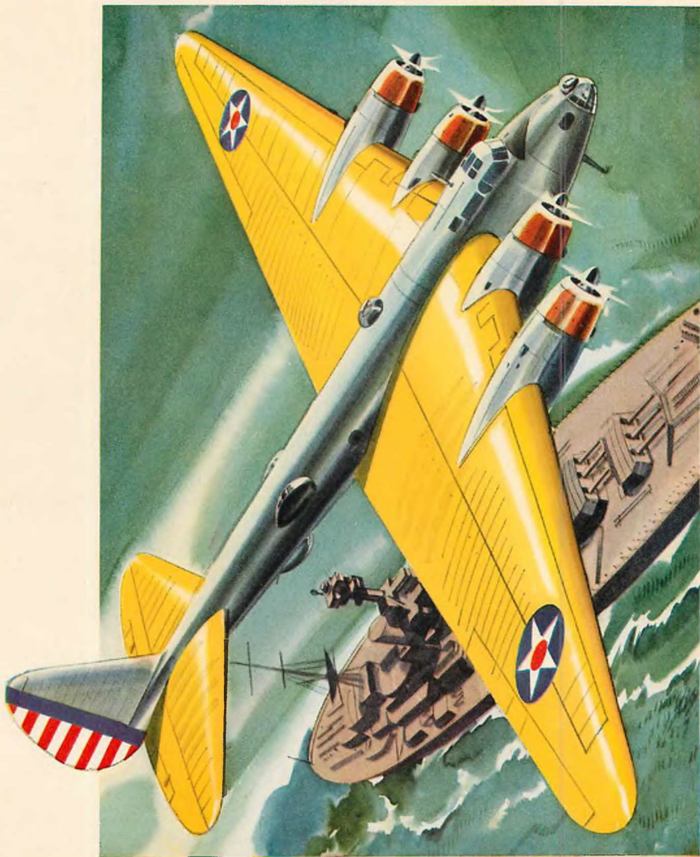
The finest bomber in the world, the Boeing YB-15. This American ship has a span of 150 feet and a length of 90 feet. It is powered with four 1,000 h.p. Pratt & Whitney Twin-Wasp Senior engines. The wings have companionways through them to the four engines.
