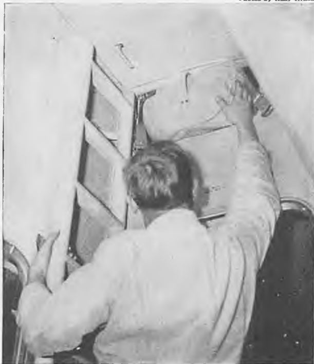
Just inside one of the roof emergency exits is stowed one of many self-inflating life rafts, each capable of holding 10 men.
