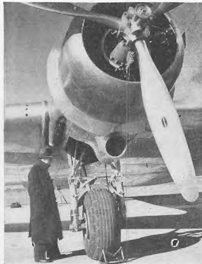
10. A typical installation: A constant-speed propeller on the Twin Wasp-powered "Mainliner."
