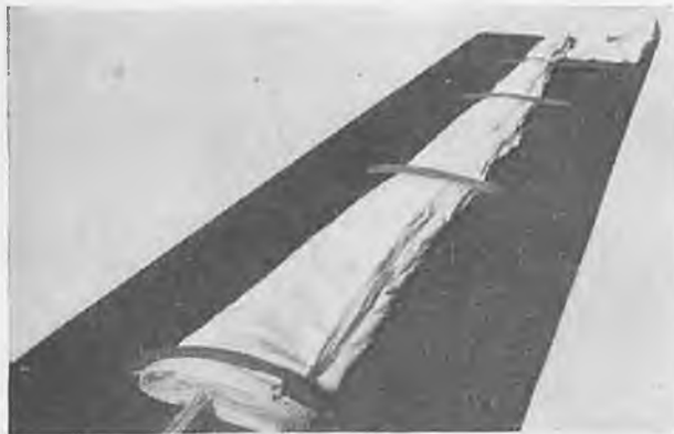
6 With both sides of canopy folded toward center, weights are used to hold down. Note the pilot 'chute at peak.
