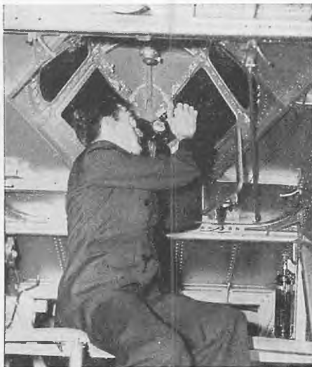
The navigator shooting the sun through the turret on top of huge cabin. This turret may also be used as emergency exit.
