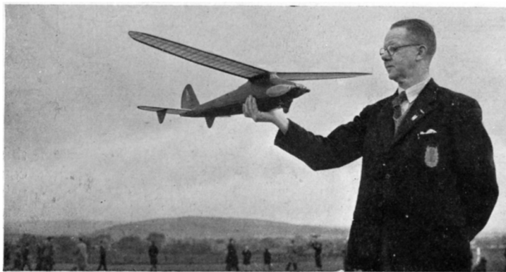
Norman Lees with his Payload Wakefield which incorporates a forward-retracting undercarriage operated by the tensioning device so that the forward shift of the centre of gravity counterbalances the rearward shift due to the folding propeller. The undercarriage is of the single leg type, hence the two stub fins on the tail to give three point support for take-off.
