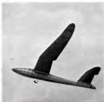
P. Vriend's remarkable "gull"-wing machine, the tail of which has a sufficiently pronounced dihedral angle to enable a fin to be dispensed with. This machine made the best performance for Holland and is one of the best "gull"-wing designs seen so far.
