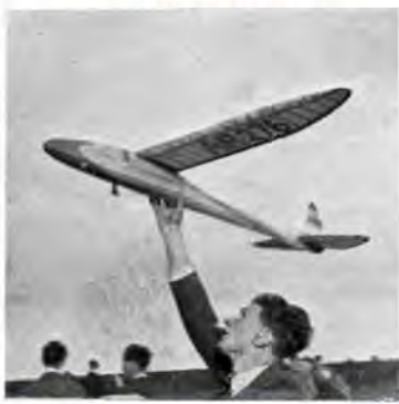
The machine flown by H. Hekking was a good performer and nicely built. It makes use of sheet-celluloid covering for the leading edge up to the main spar—a form of construction which finds considerable favour in Holland.
