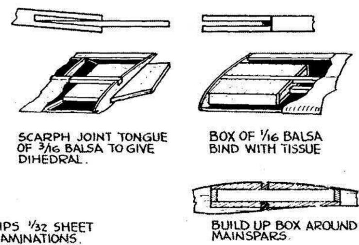
FOR MODELS ABOVE 4' SPAN IT IS SUGGESTED 1/ THAT THE TAIL PLANE BE STRUT BRACED, AS BELOW. 2/ THE FALSE SPAR METHOD OF WING JOINT IS USED. THIS MEANS TWO Balsa "BOXES" IN EACH WING SECTION TO BE JOINED INTO WHICH ARE PUSHED FALSE SPARS OF HARDWOOD OR Balsa STEAMED TO DIHEDRAL. IN THE EVENT OF A CRASH THESE SPARS WILL BREAK.
