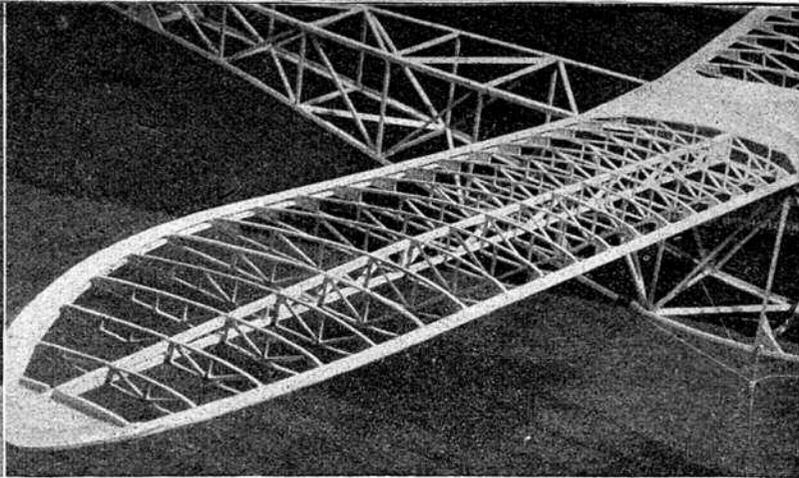
*This interesting model of 64 in. span was designed and built by Messrs. Hogan and Nelson of the Bristol & West M.A.C. An enormous amount of detail work is incorporated, particularly in the wings, and makes this model an outstanding example of fine workmanship. The only weak point appears to be the wire undercarriage, which hardly seems appropriate on a model of this size. (Note copy of the Aeromodeller for comparison.)*
