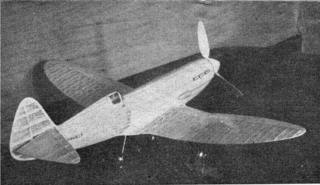
tube must be built round cardboard formers first; correct alignment is essential as any warp or twist may be imparted to the fuselage. The sheet should be wetted, the formers inserted and the whole weighted down between two flat surfaces. The joint must be lined by a strip of  $\frac{1}{4}$  in. by  $\frac{1}{32}$  in. on the *outside* and both sides covered with a strip of tissue. The whole tube should then be covered with tissue. The rear end has to be cut away in various places
