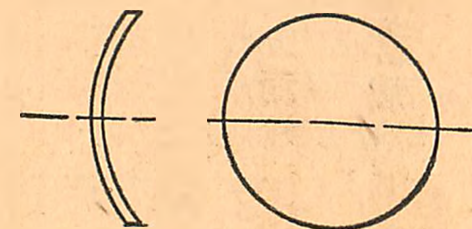
CYLINDER HEAD FORMED FROM 1/32 SHEET BRASS TO SUIT CYLINDER TWO REQ.
