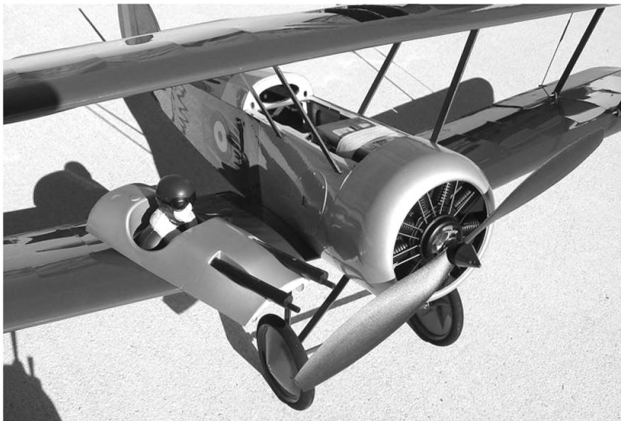
Access to the battery is easy, but actually connecting and disconnecting the battery is tedious for big hands in the limited space under the wing.
