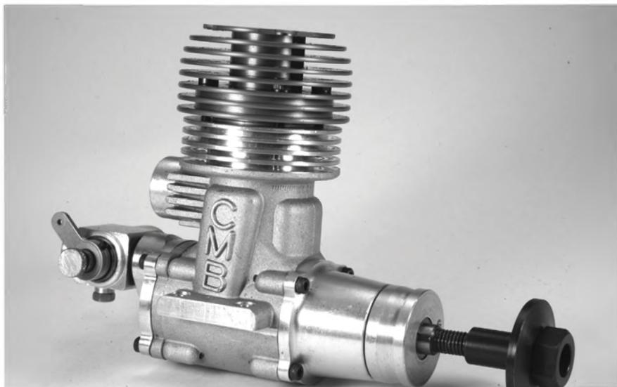
**Photo 7:** This CMB 80 ducted fan engine has the potential to rev very high with a fan or flywheel, but it still runs very nicely with applicable size normal props, which is what I used when I tested it for a review.
