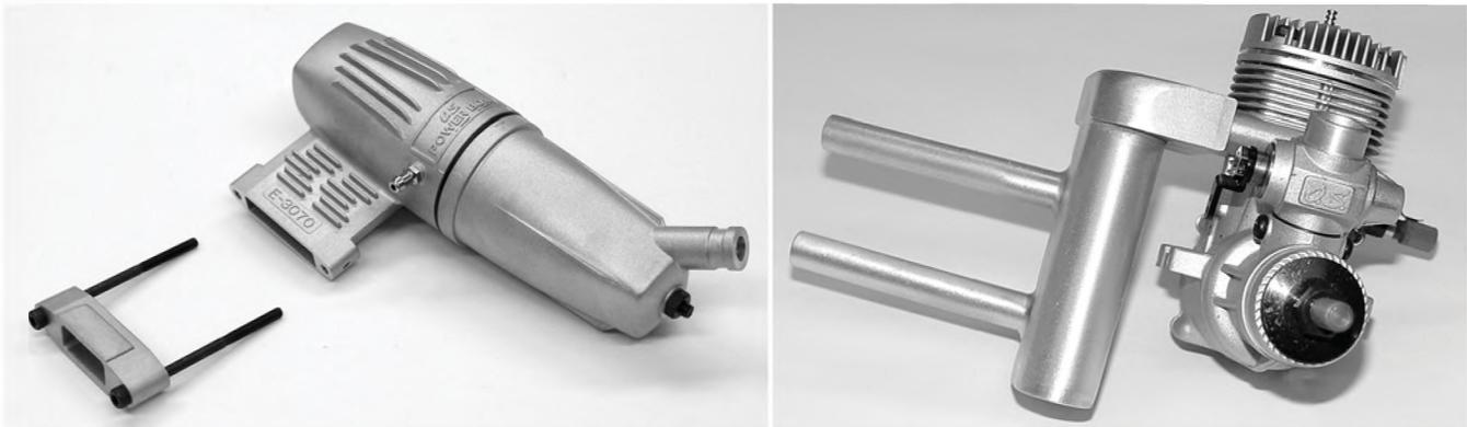
**Left:** With one extension, the O.S. .46AX muffler will work, but the cowl will require more cutting, and the firewall will have to be modified. **At right is the \$36 Bison Pitts-style muffler. It makes assembly easier, and makes the completed model look nicer. I later shortened the tubes by about half. The noise level is higher than the O.S. muffler, but is still acceptable.**
