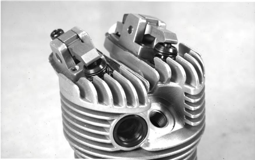
**Photo 5:** This is how the rockers appear when both valves are fully closed.
