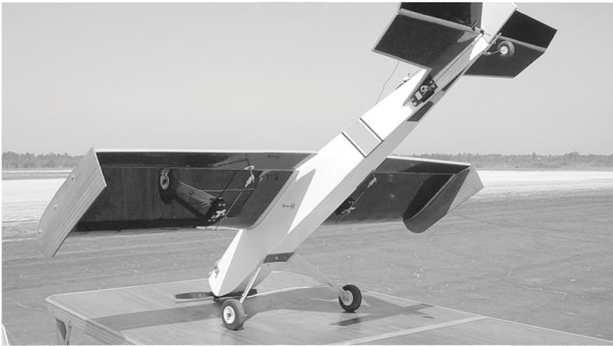
**Photo 2: Ed's Little Stick with downward end plates to stop roll with rudder.**
