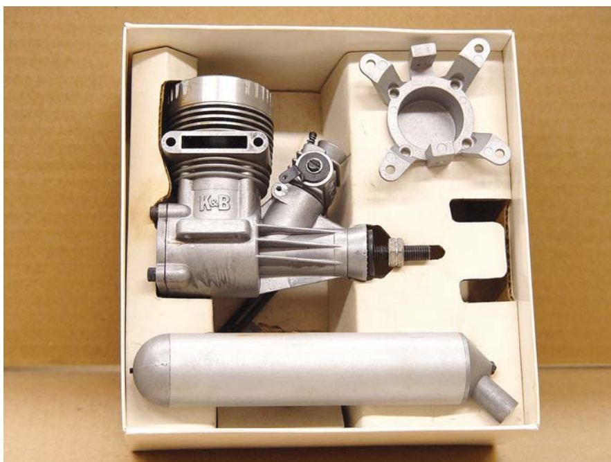
Here's my one and only "famous engine". It's the first K&B Sportster 45 to leave K&B's possession, and it turned out to be a final prototype, having coarse-thread fasteners instead of the fine-thread screws used in the production engines. It also performs far better than the production engines ever did.
