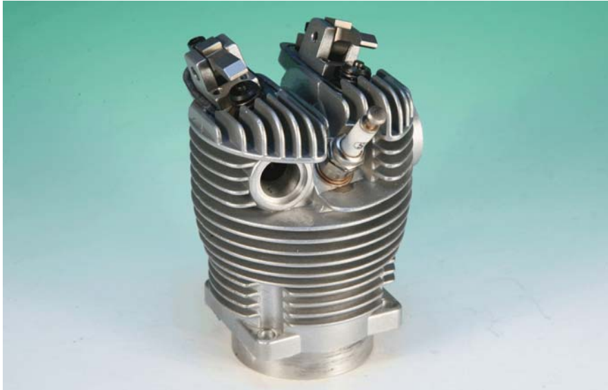
Photo 4 shows the one-piece cylinder and cylinder head. No head gasket here!
