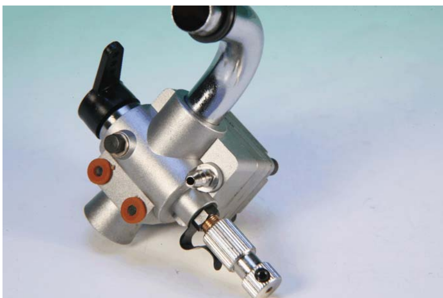
Photo 7: The normally hidden side of the Saito FG-20 carburetor. Note the heat insulators around the mounting screws, to help keep the carb cool.
