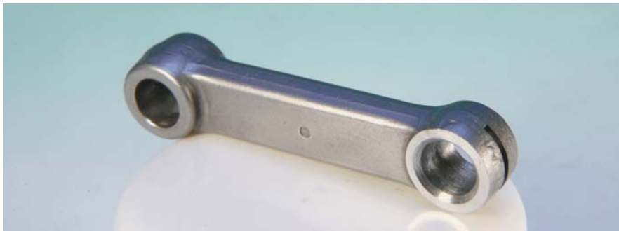
Photo 3: The Saito FG-20 connecting rod.
