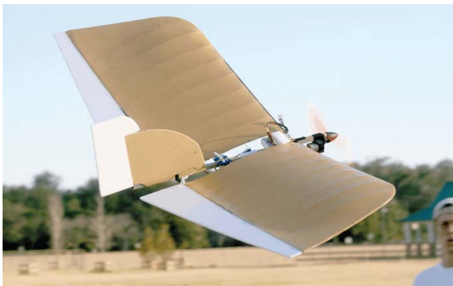
Photo1: The ORB (see text) is a homemade flying wing adapted from the surviving parts of an abused Ikarus Bleriot foam slow flyer. Note that it uses rudder/elevator controls instead of elevons, which are standard on flying wings. Small electrics are ideal for this sort of tinkering. (Lewis Dunn photo)
