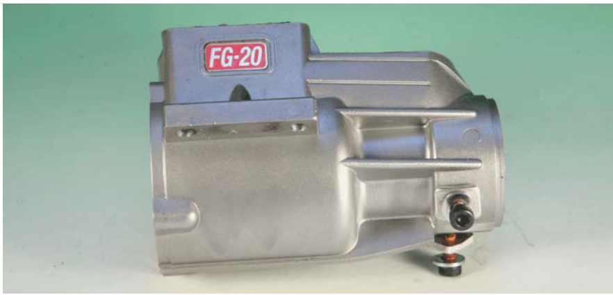
Photo 8: The Saito FG-20 has a beautiful cast aluminum crankcase. (Editor's Note: Brian particularly likes crankcases because he's an old crank!)
