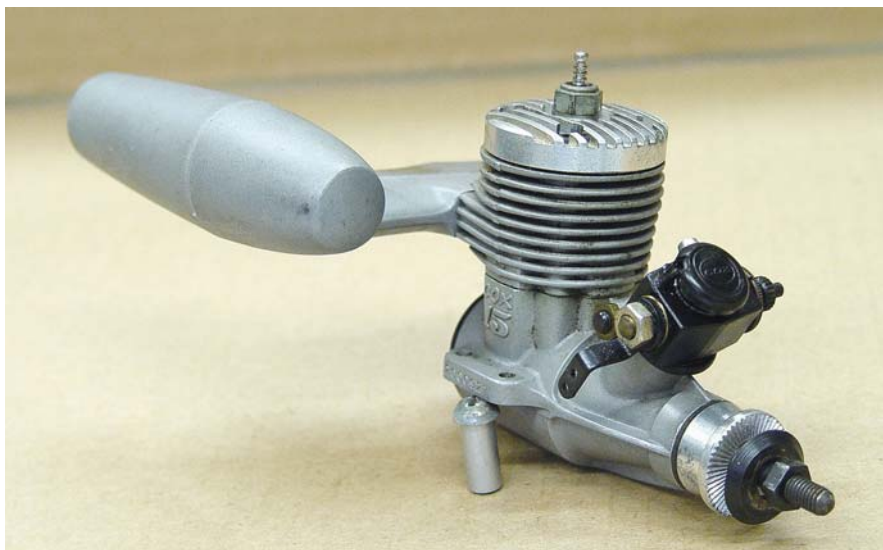
This old K&B Cox .15 was limited to small, speed props, but man oh man did it scream! Its very unusual rear-mount muffler is loud, but it lets the power out!
