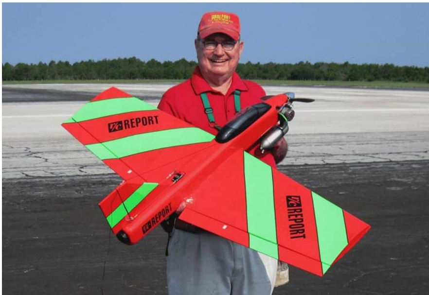
Photo 5: Ed and his Bill Evans' design Pole Star flying wing. Ed uses a Tower .75 for power, making the Star very fast.
