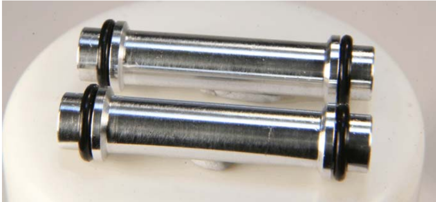
Photo 19: Previously the pushrod covers were formed from stainless tube. The new style is fully machined aluminum alloy.
