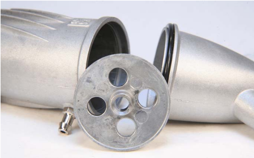
Photo 16: Effective but not overly restrictive baffle for the exhaust system.
