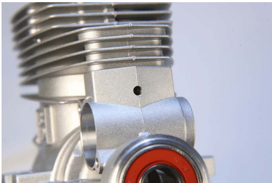
Photo 11: Handy hole in the front for removing the wrist pin from the piston and connecting rod.
