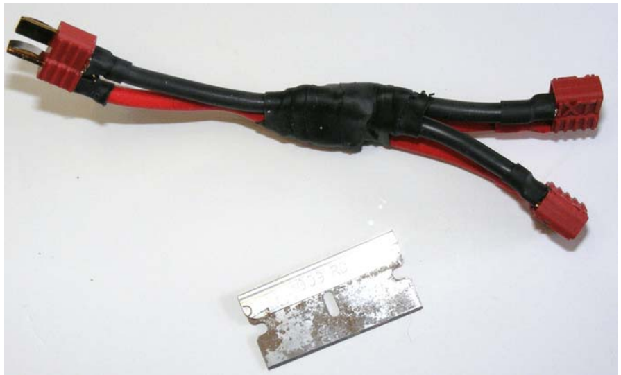
Photo 1: My parallel adapter for two wattmeter inputs
