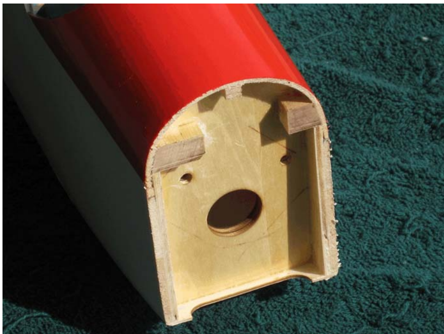
Photo 6 shows the Rascal nose with the cowl and hardwood beam mounts cut off.
