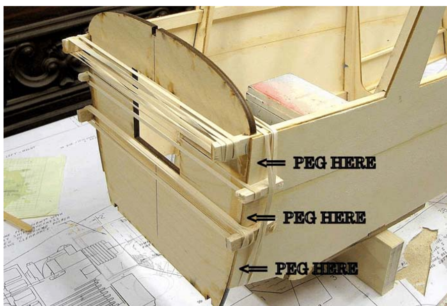
Photo 3: Typical peg locations on a fuselage-to-firewall joint.
