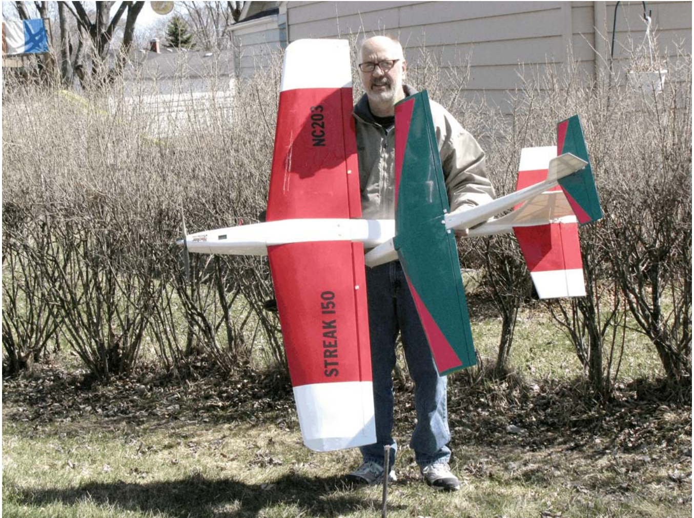
Photo 1: Dennis Vollrath shows off his scratch-built Streak 150 along with its inspiration, a Great Planes Electrostreak. Dennis powers the Streak 150 with a Hacker brushless motor and A123 batteries.
