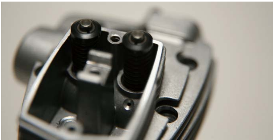
Photo 7: All the oil gets sucked down this small drain hole.
