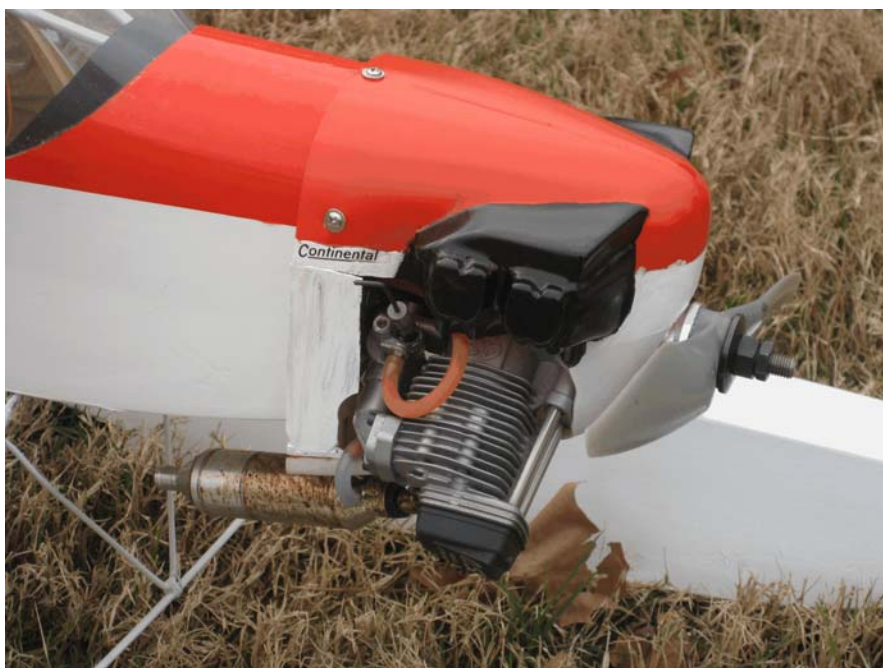
Photo 7: The OS .70 Surpass mounted 45° down, under a fiberglass Cub cowl.
