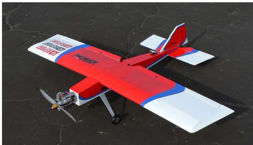
Photo 1: Ed's OS .55AX powered Ultra Stick 40 with 3° of anhedral in each wing panel.
