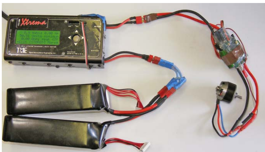
Photo 3: A basic single wattmeter setup.
