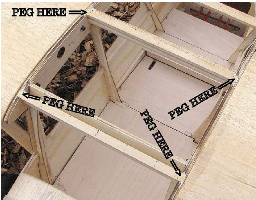
Photo 5: Location of music wire pegs to reinforce the critical wing-to-fuselage joint.
