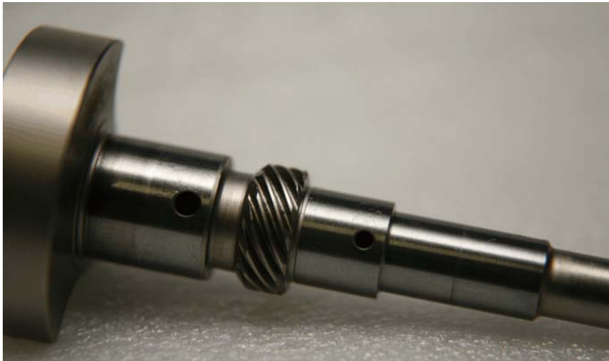
Photo 9: Acting as a centrifugal pump, the crankshaft flings the oil on its upward path.
