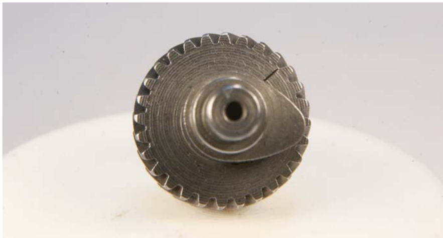
Photo 14: Out with the dot, in with the slot: the new timing mark on the cam gear.
