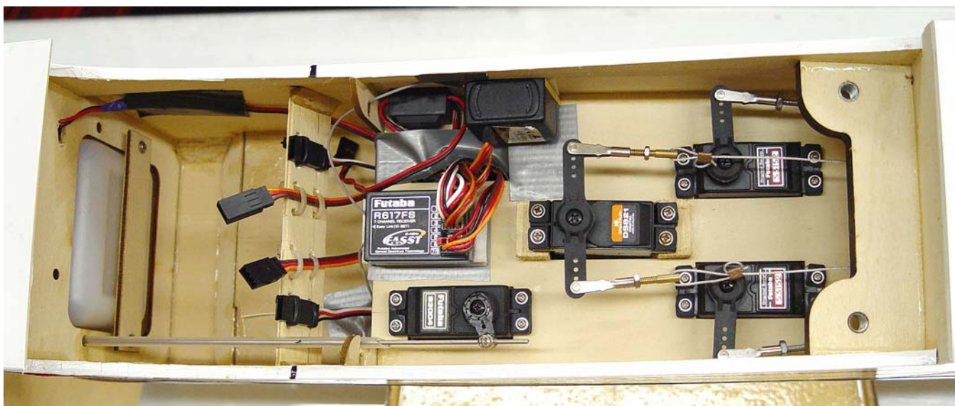
Photo 3 shows the radio compartment in my Goldberg Tiger 120, with the servos installed where the instructions suggested. Had I moved all those servos far to the front, I could have prevented the need for so much dead lead in the nose. Warning: Photo 4 is ugly and unsuitable for weak stomachs.
