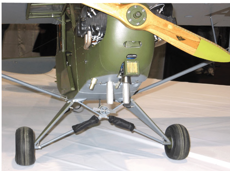
Front view showing details of landing gear, engine, and prop
