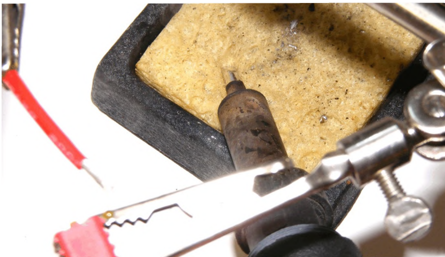
Photo 3: A quick wipe on the sponge cleaned the iron.
