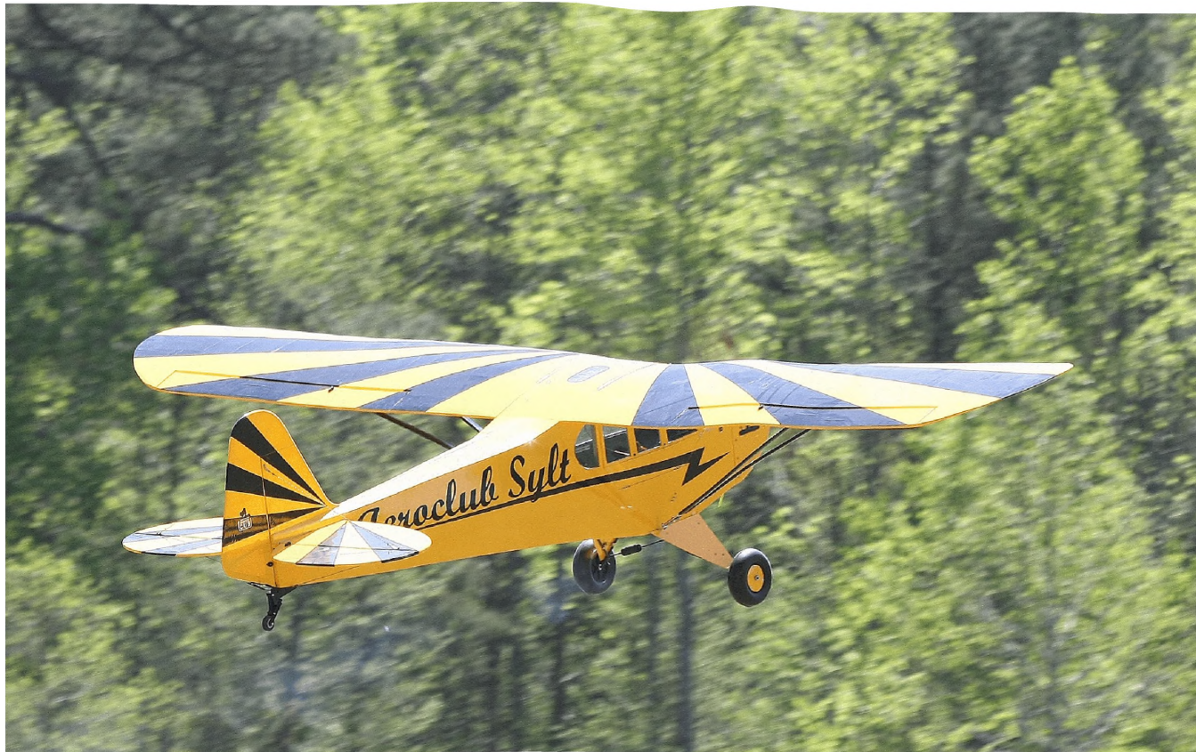
Photo 6: Gotz Vogelsang's 1/3 scale Clipped Wing Cub has a 120" span, weighs about 28 lbs. with its DA-85 gas engine and Menz 26x10 prop, and uses a Spektrum radio with Hitec digital servos and dual 5-cell batteries.
