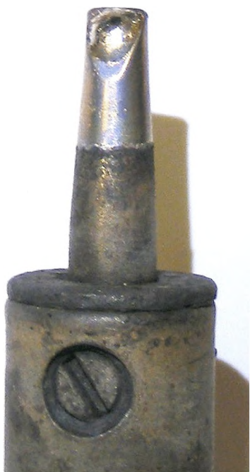
Photo 6: The clean iron with a small drop of solder on the tip for tinning the connector.
