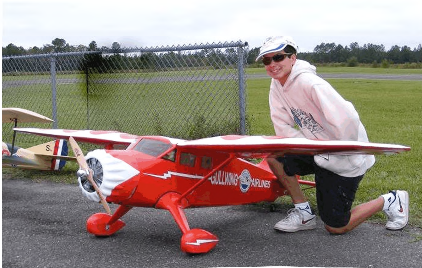
Photo 2: Here's John's Top Flite Stinson Reliant SR-9 built from a BIY kit. This one uses a Quadra 42 gas engine and a Futaba FASST radio system.
