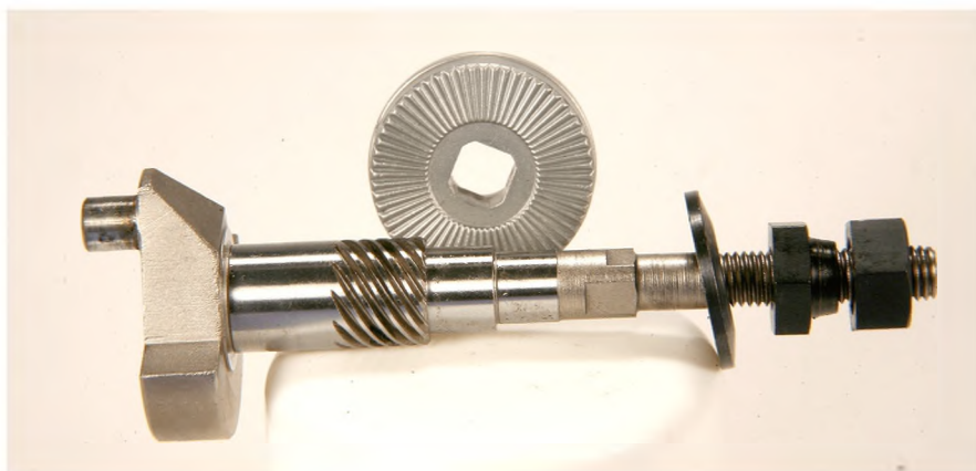
The short side of the square-length is to maintain a timing reference.
