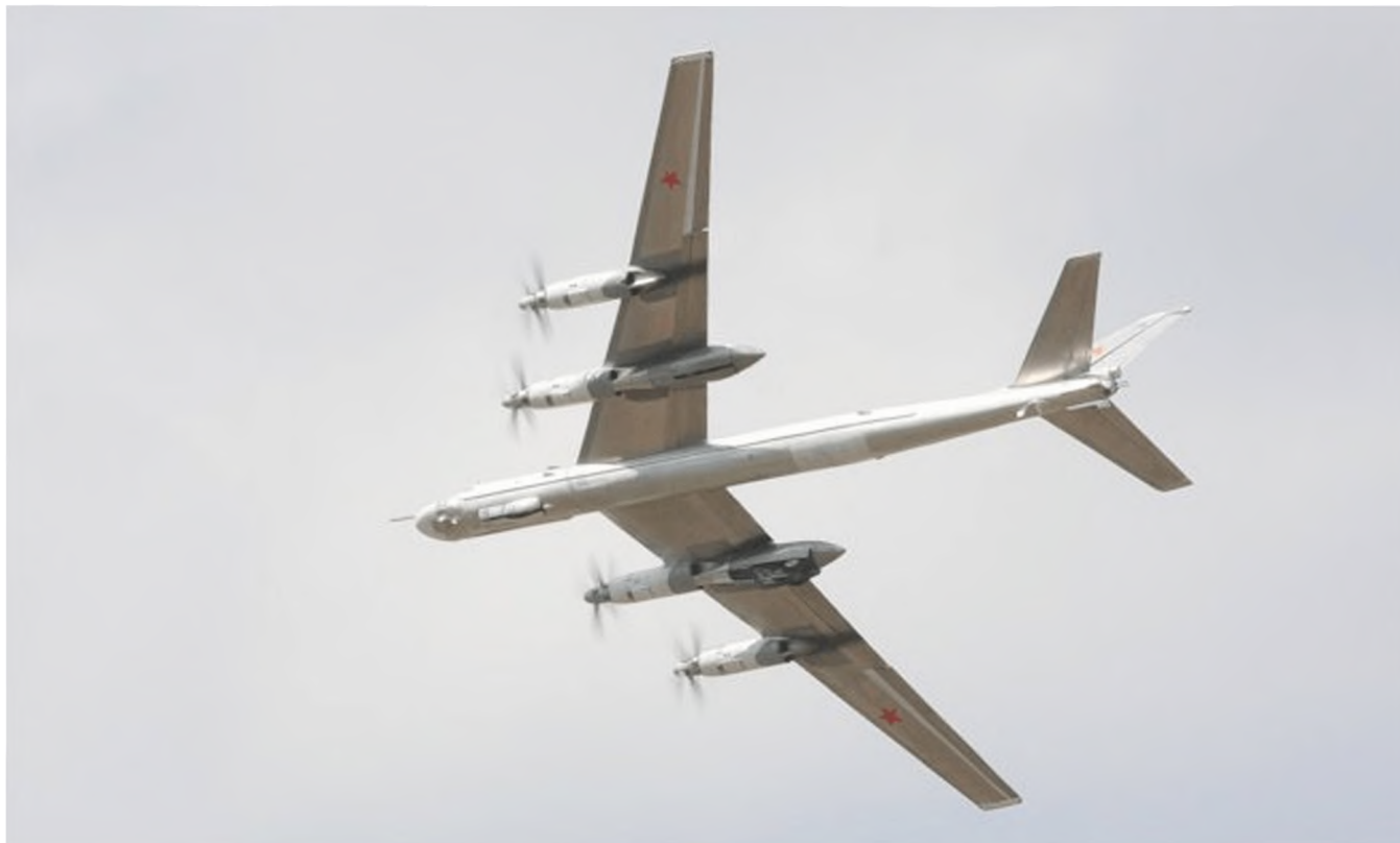
Photo 34: Underside of the electric powered Bear with counter rotating props
