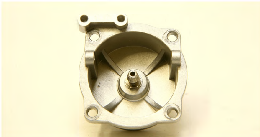
With the breather nipple in the center of the rear cover, there's a safety margin area underneath for extra low end lubrication.
