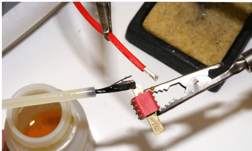
Photo 5: I add small drop of liquid flux to the wire and connector.
