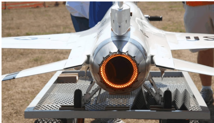
Photo 22: Here's the Falcon's LED simulated afterburner.
