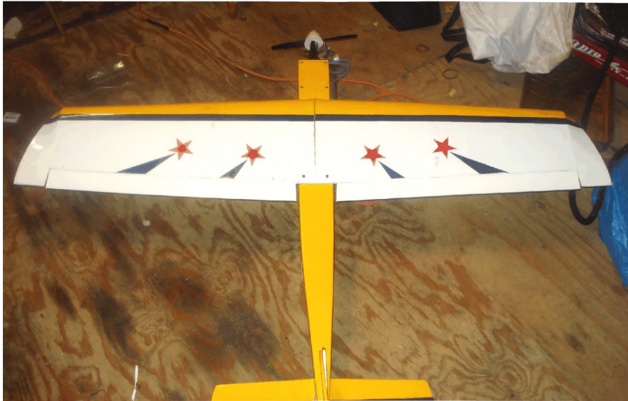
Photo 2: ...but not with the new, shorter and narrower ailerons.
