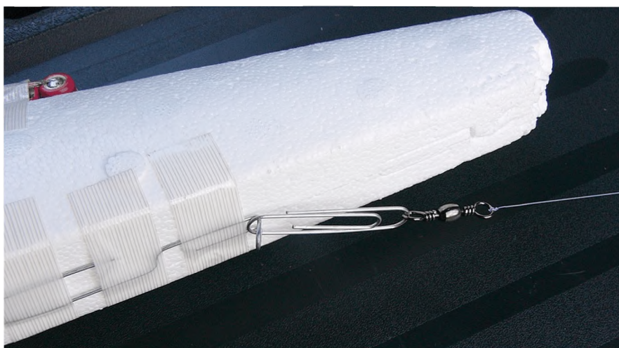
Photo 5: More paperclips are used on the glider's end of the tow line. The passive "hook and loop" attachment system seems to work well.
