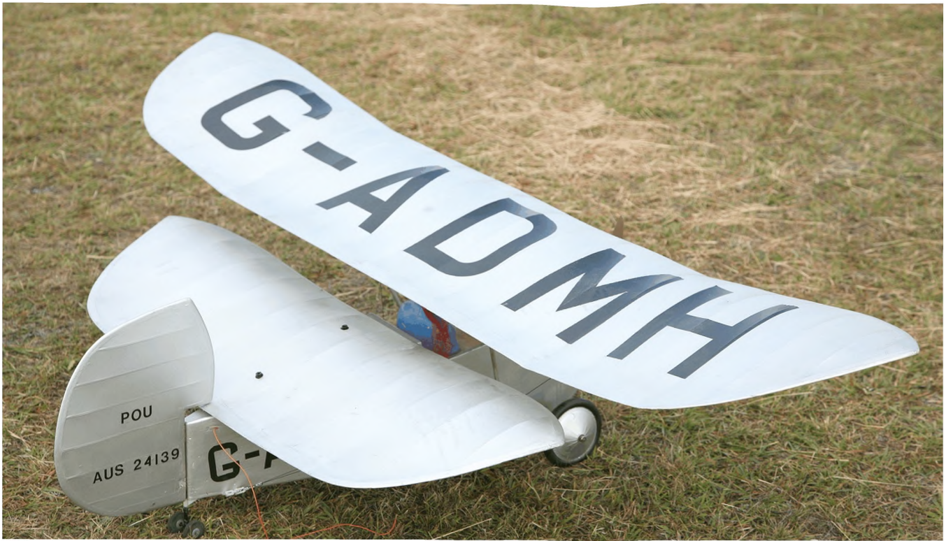
Photo 4: Here's an economy biplane. You save on horizontal stabilizers! Actually it's a scale model of a French Pou du Ciel (Flying Flea), a popular home-built tailless biplane design of the 1930's.
