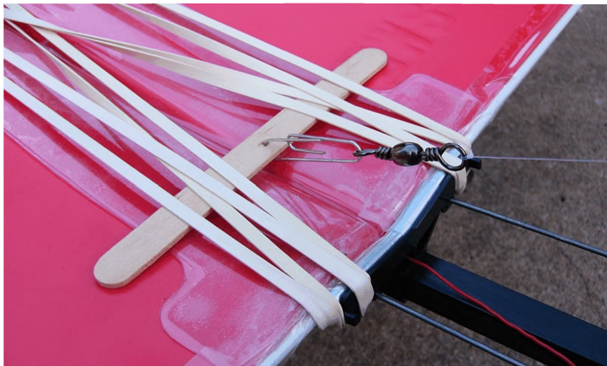
Photo 4: Common household items are used in the Slow Tow's tow line. A craft stick and paperclip attach the line to the GWS Slow Stick tug. Don't forget the swivel!
