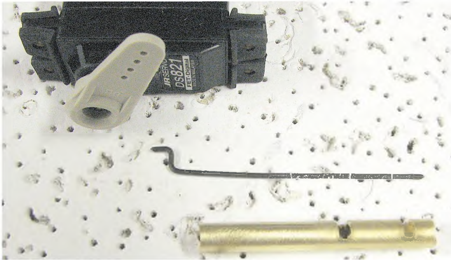
Photo 3: Parts of release mechanism inside fuselage
