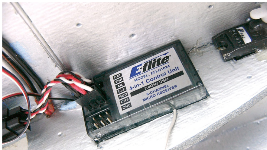
Photo 2: I was hoping that the differential-thrust yaw control inherent to this heli 4-in-1 unit would have more control authority, but even so, the Lil-Lightning is still a hoot to fly in calm airs.
