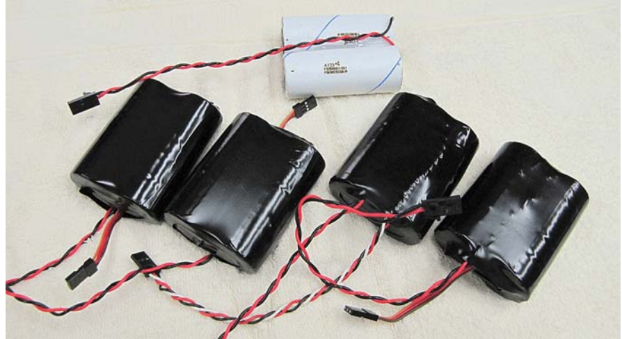
Photo 2: Homemade A123 batteries with output and balancing leads
