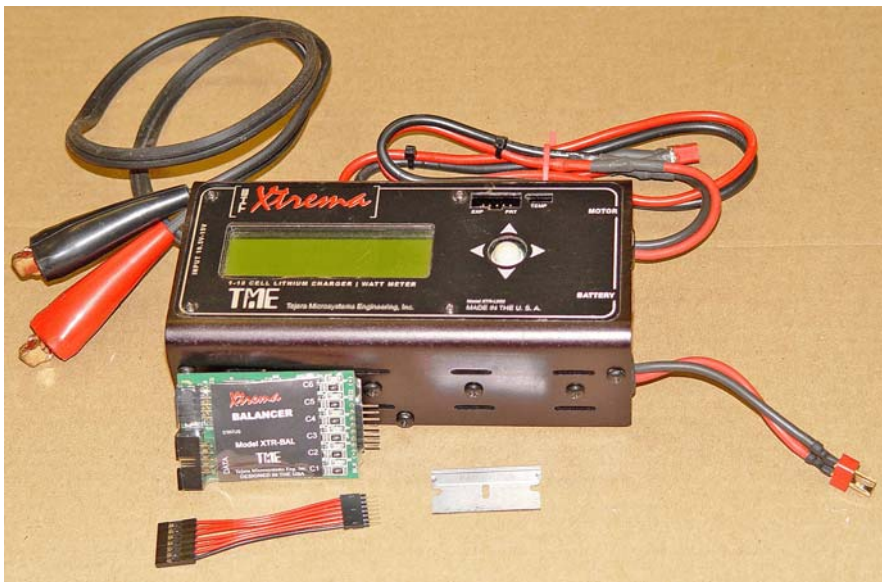
Photo 3b: The little TME Xtrema Balancer, shown with the Xtrema charger and an optional cable adapter. Razor shown for size reference.
