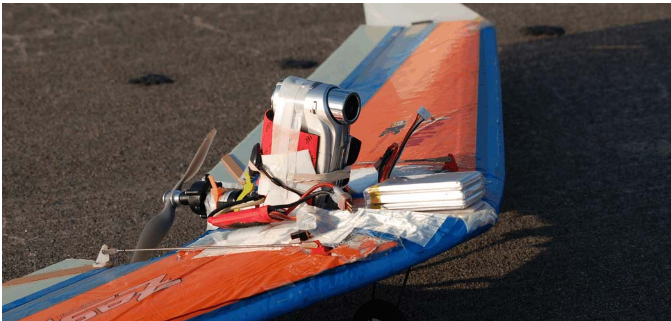
Photo 3: The Aiptek A-HD+ 1080P wasn't so easy to use on the Zagi. It fit my homemade mount just fine, but the rubber bands would invariably squeeze one of the buttons on the camera and foil the filming. I eventually gave up and used the Aiptek on different airplanes with less anaconda-like mounts.
