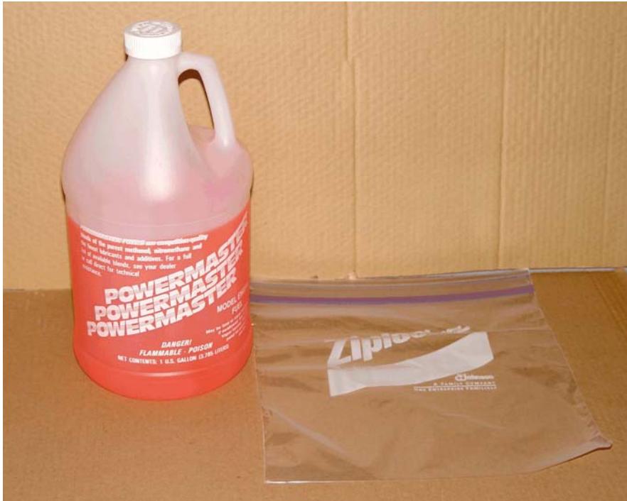
The problem (a less than full bottle of fuel containing moist air) and one possible solution (an air tight and fuel resistant Zip-Loc storage bag from which air can be easily expelled).
