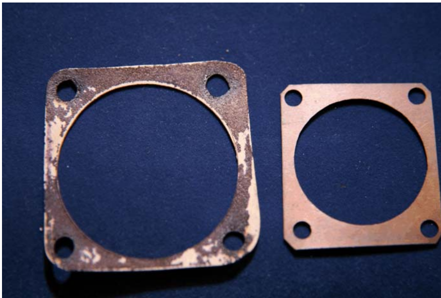
Photo 1: Saito base shims made from very hard gasket card on the left, and bronze sheet metal on the right.
