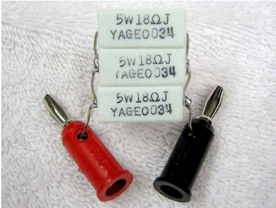
Photo 5: Homemade 1 Amp load resistor for checking an A123 battery's voltage under load
