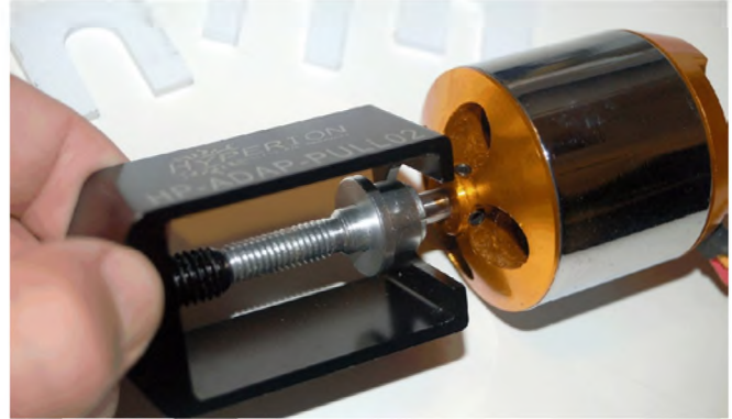
Photo 4: Hyperion makes a useful tool for removing sticky drive washers from collets. I also made several plastic adapters so I can use this tool on smaller collets.
