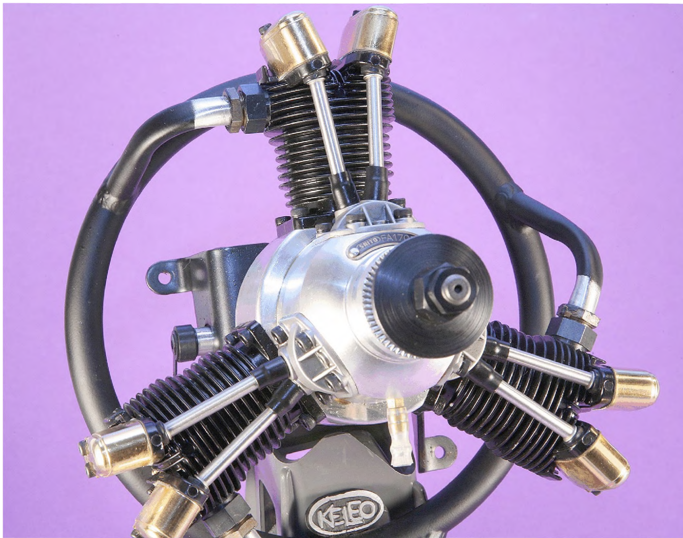
Photo 5: My Saito 170 fitted with a twin outlet Keleo collector ring exhaust.
