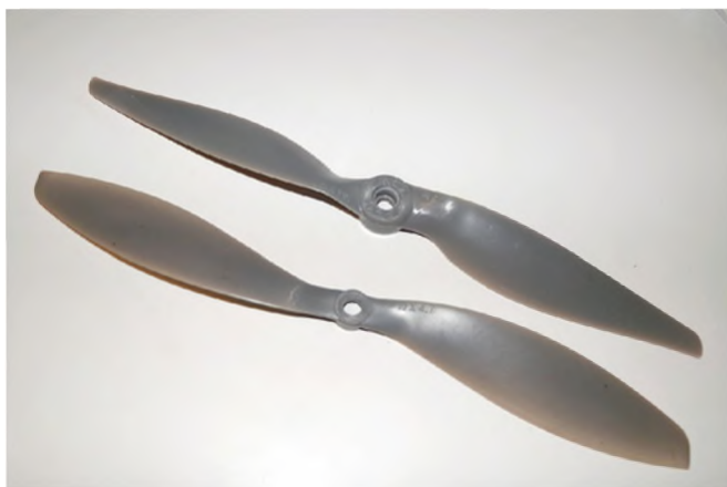
Photo 7: These are both 10" electric props from APC. The standard version on top can tolerate much higher RPM than the Slow Flyer version below. The latter is showing some light-colored stress marks on the left blade, so it's time for a replacement.
