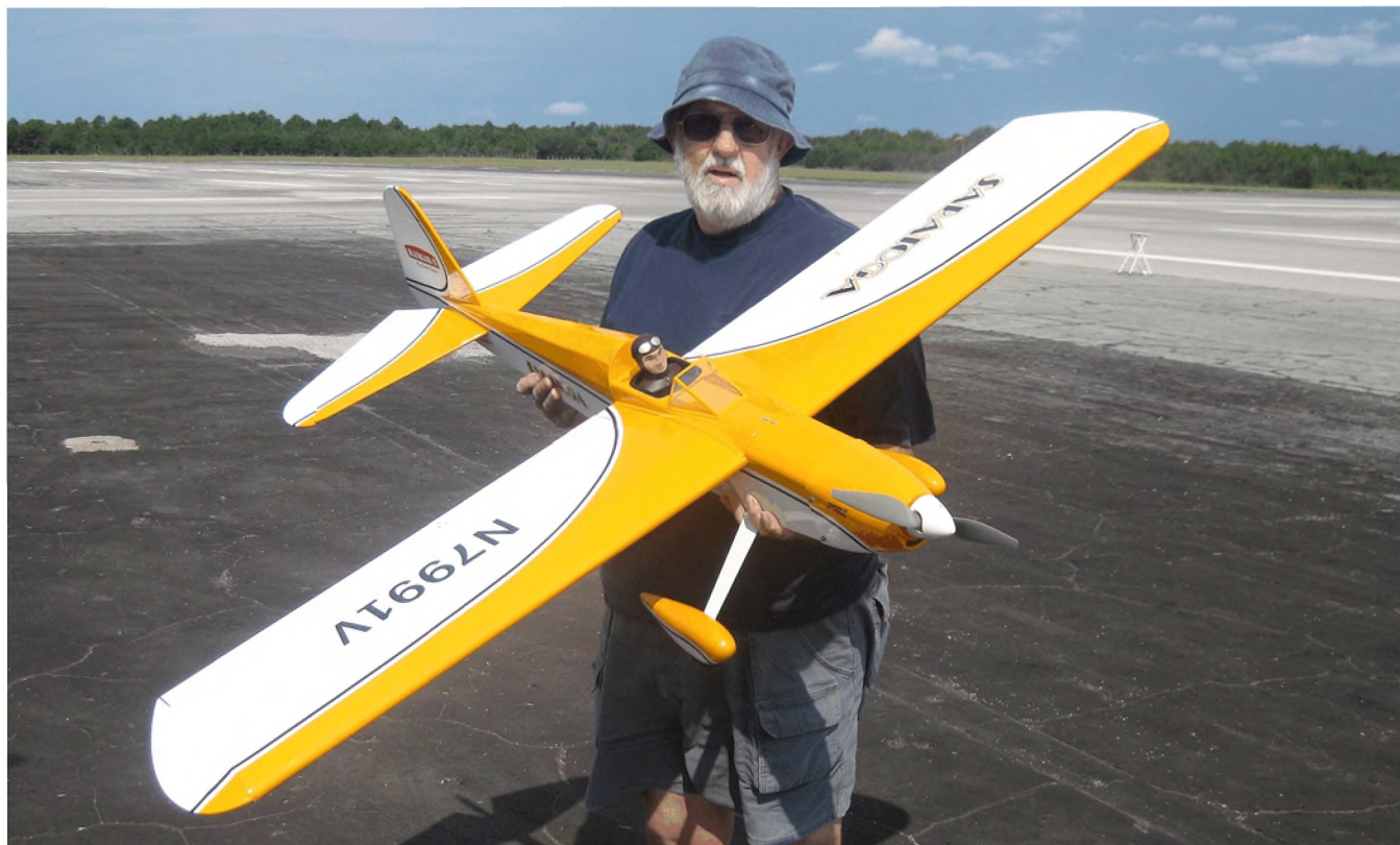
Photo 1: Don Warren and his new Hangar 9 "Saratoga" with electric power. I've flown this plane and it is very smooth and steady. Don has an E-flite Power 46 motor in it, with a 5-cell LiPo battery. Personally, I'd like to see an OS .55AX in it. I like engine noise, and after many years of flying USAF jets, my hearing is shot anyway.
