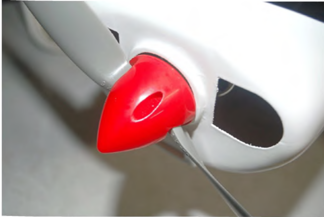
Photo 5: Standard nylon spinners designed for glow engines are often tough to use on electrics. This model from Hyperion is one of numerous spinners made exclusively for electrics.
