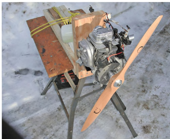
Photo 3: Here the GX35 has been converted and is ready for testing. It performs very nicely, swinging a 22x6 prop at 5460 RPM. Both engines actually run close to the same speed.
