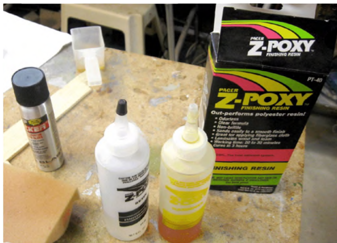
Photo 1: Zap finishing resin is used to attach the gloss cloth
