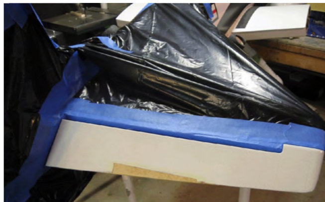
Photo 2: Elevator ready for primer and surface detail. Note use of black garbage bags for masking. No over-spray can get past the plastic.
