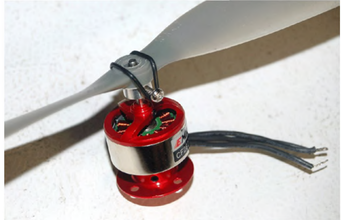
Photo 2: One particularly useful type of set screw prop adapter is the "wobbly" prop saver. It uses an o-ring to absorb soft impacts and protect the motor shaft and prop.
