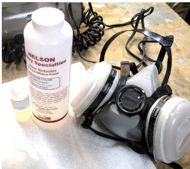
Photo 7: Nelson's Clear was used to protect and fuel proof the paint. Notice the use of a charcoal-filter respirator, and gloves for protection.
