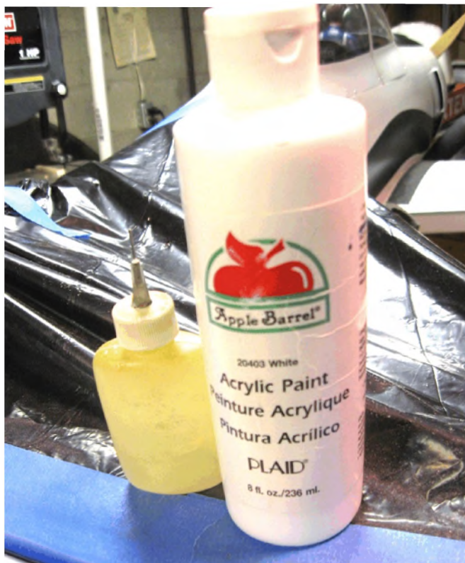
Photo 4: Acrylic water based paint used to create the exposed rivets. It comes in a variety of colors, even aluminum. If you plan on weathering and sanding through the color, it will look like bare metal rivets.
