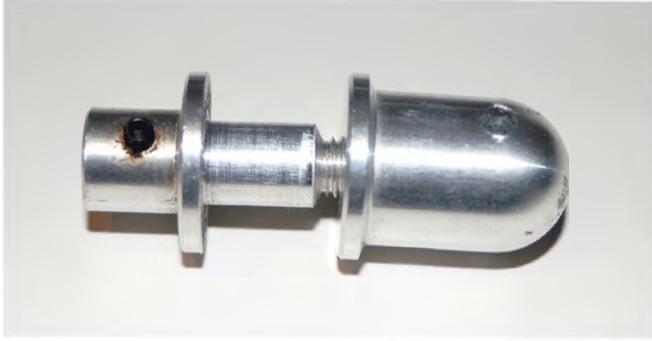
Photo 1: I wouldn't go so far as to say that set screw type prop adapters are evil. Let's just say that they aren't my first choice when it comes to airscrew fastening.
