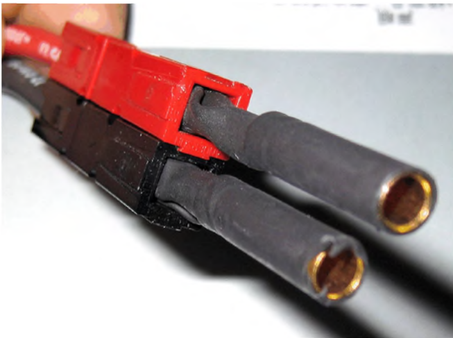
Photo 6: My Anderson Power Poles/banana plugs adapter
