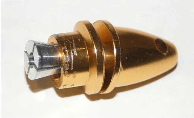
Photo 3: Collet prop adapters are my preferred method of propeller attachment. They center perfectly and have a tight grip on the motor shaft. Note the scarred drive washer caused by using pliers for removal. There is a better way.
