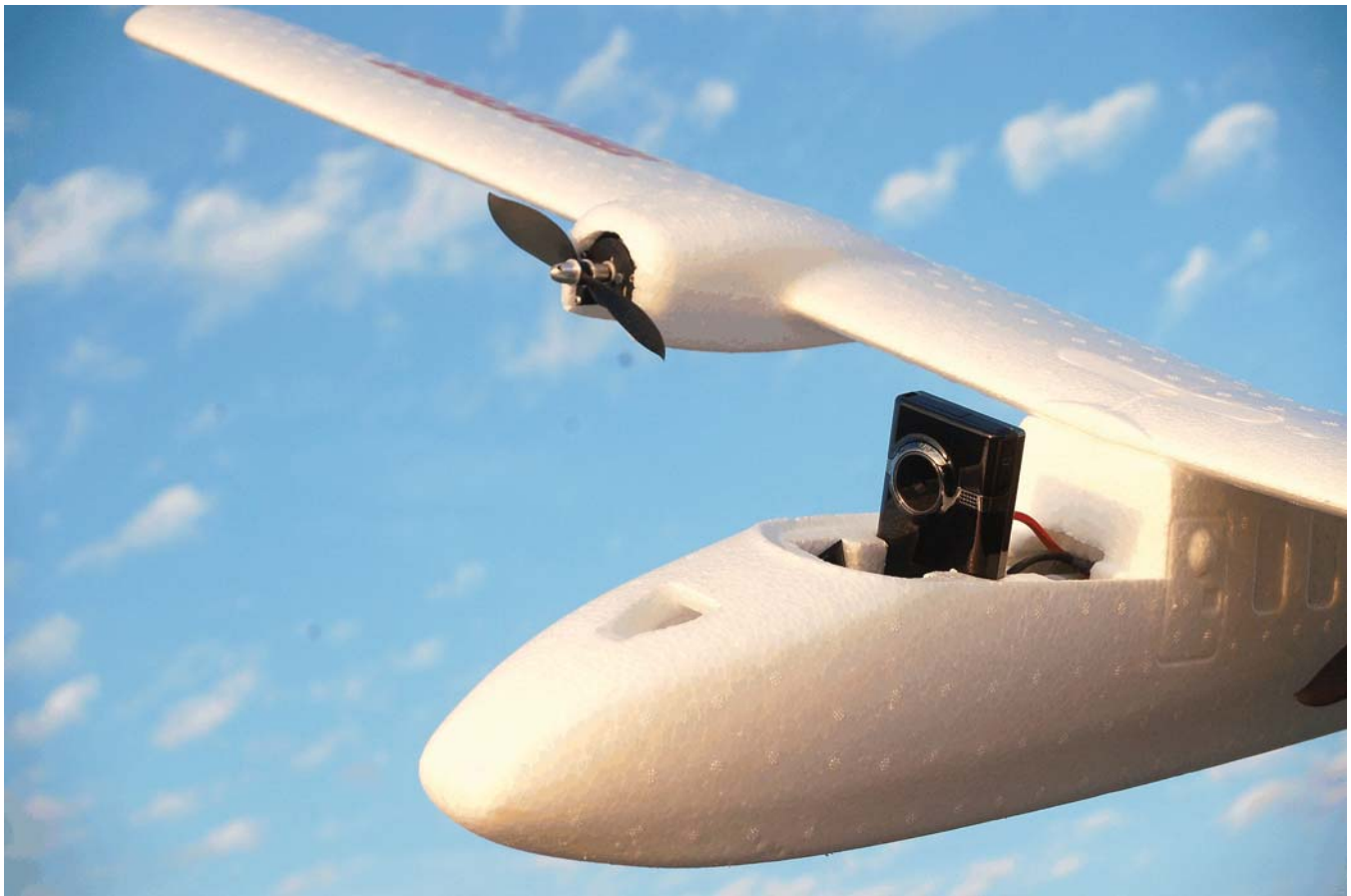
Photo 2: A simple slot cut into the foam fuselage of my Multiplex Twinstar II keeps a tight grip on the Mino HD. Note the slight downward angle of the camera that provides more ground and less sky in the picture. (Fitz Walker photo)
