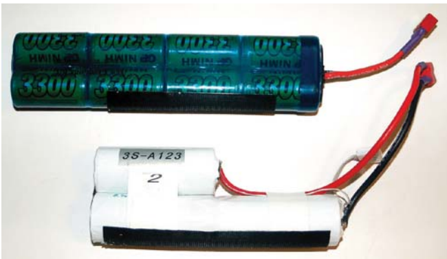
Photo 5: My 3-cell A123 battery (bottom) provides about the same voltage as an 8-cell NiMH battery, but it is a lot lighter. The unique shape of this pack is solely to accommodate my onboard video camera.
