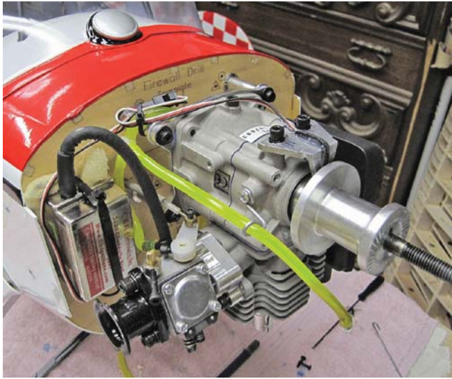
Photo 4: Complete installation of the CH Electronics RCEXL ignition system
