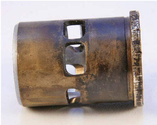
Photo 7: This liner suffered terrible rim damage, and is now oval from an attack with one of the gripping tools.
