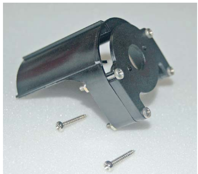
Photo 3: The screws included with the plastic motor mounts were too small, so I replaced them with 2-56 bolts and nuts.
