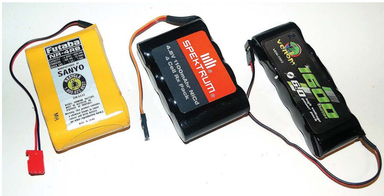
Photo 2: Switching to a 5-cell receiver battery (right) will provide a little breathing room to help avoid brownouts, but a properly charged 4-cell battery (left and center) will work just fine with 2.4 GHz radio systems.
