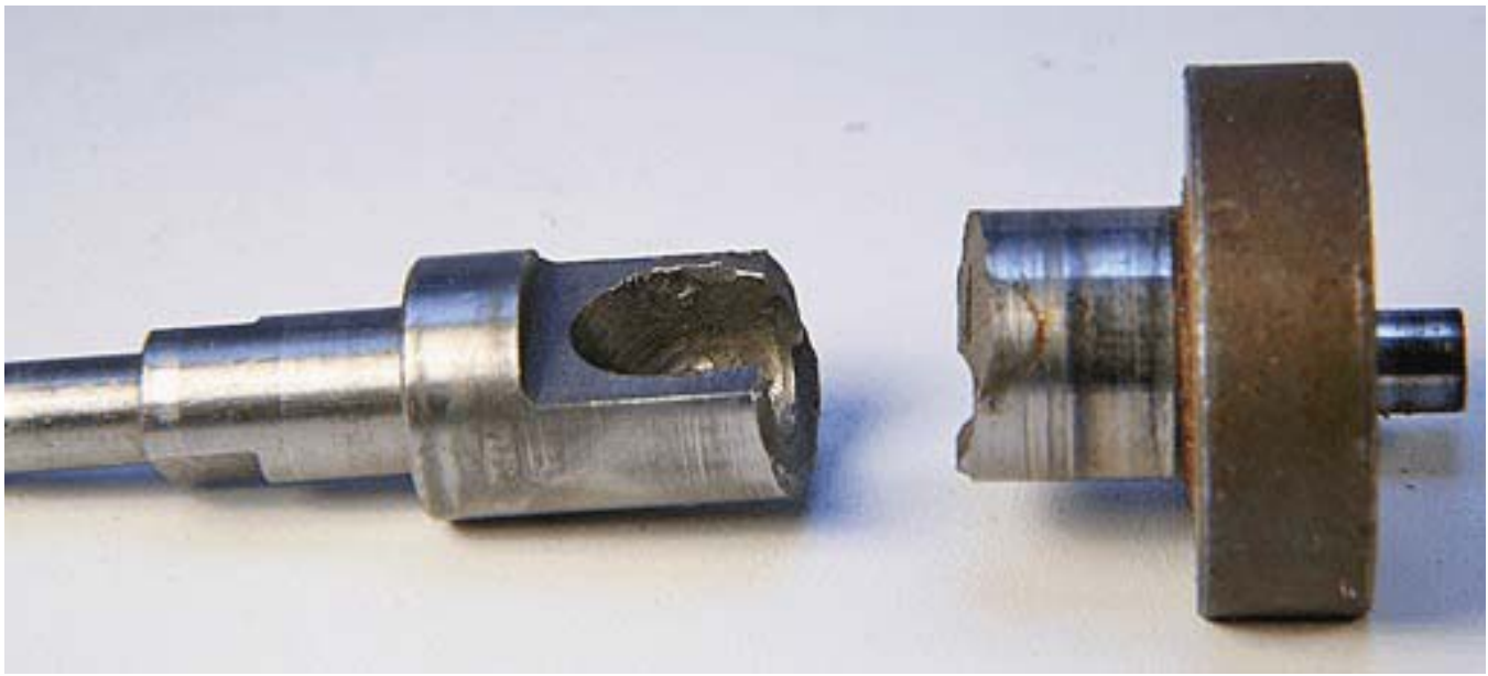
Photo 8: In the port of this crankshaft you can see the damage from the inserted screwdriver that led to the eventual breakage.
