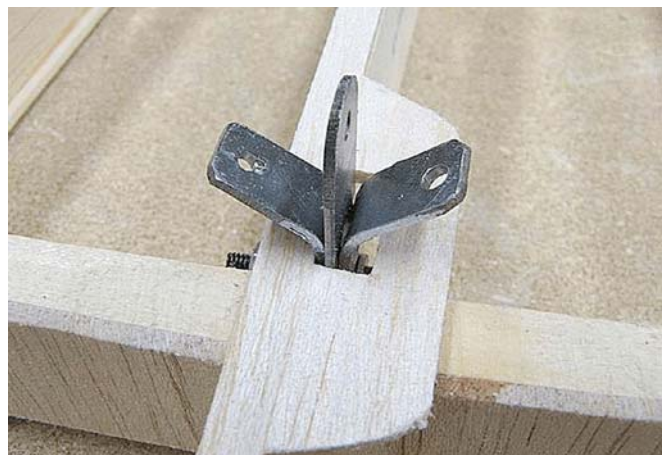
Photo 6: Brackets installed on DH-4 wings
