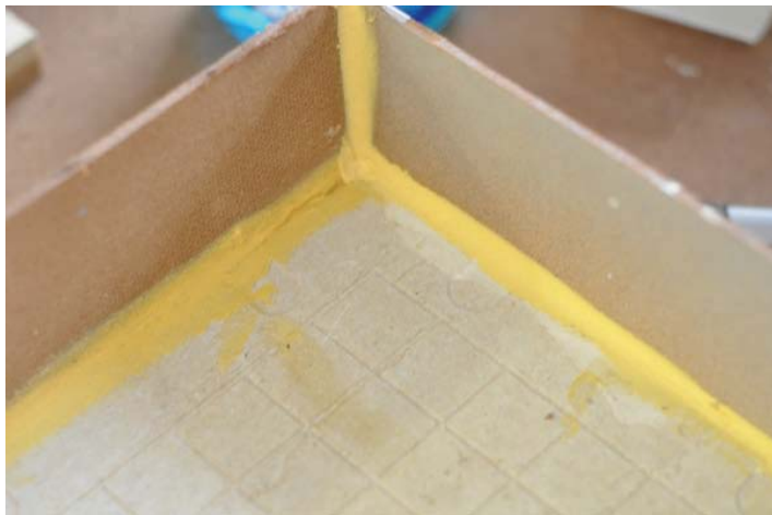
Photo 4: Sides glued on with fire caulking
