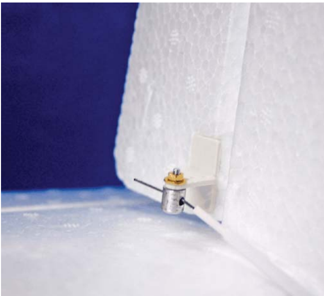
Photo 1: I inverted the pushrod connector on the rudder horn to reduce the curvature of the pushrod. Now, I have to stick the wrench through the stabilizer to get to the set screw.
