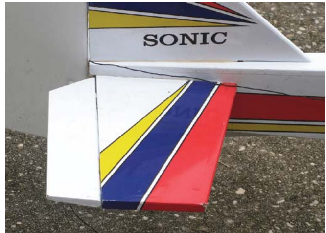
Photo 7: Elevator with mix on and left rudder
