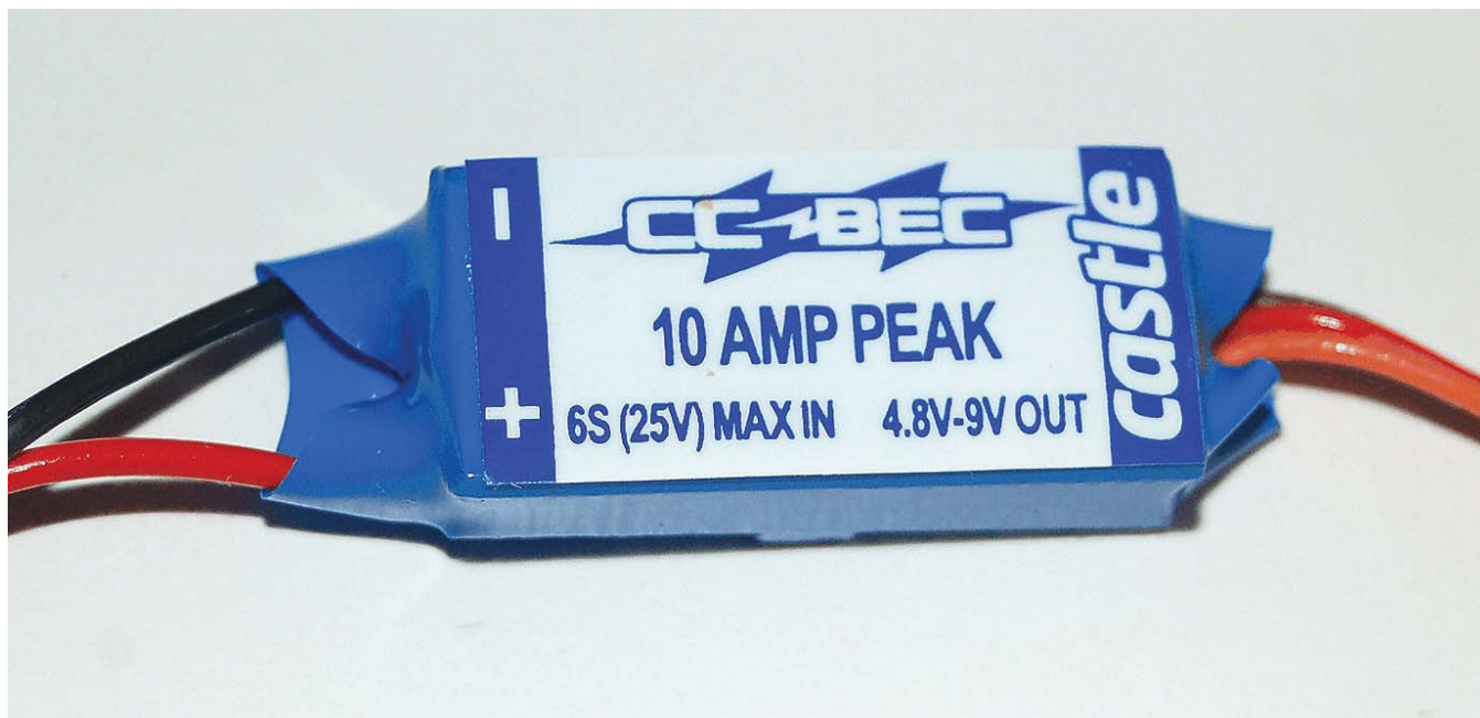
Photo 3: A discrete switch-mode BEC, such as this CC-BEC from Castle Creations, is better able to provide reliable power to your receiver than the linear BEC built-in most ESC's.
