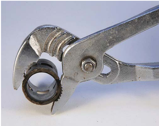
Photo 5: Multi-grips can exert incredible pressure, and the teeth can do a lot of damage.
