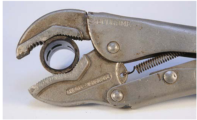
Photo 6: Vice-grips have an even a stronger grip, and can distort or crush things easily.
