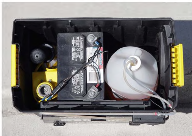
Photo 4: Here's a better look at the contents and arrangement of the lower section which is my "Fuel and Power" module. The fuel pump is mounted on the front face.
