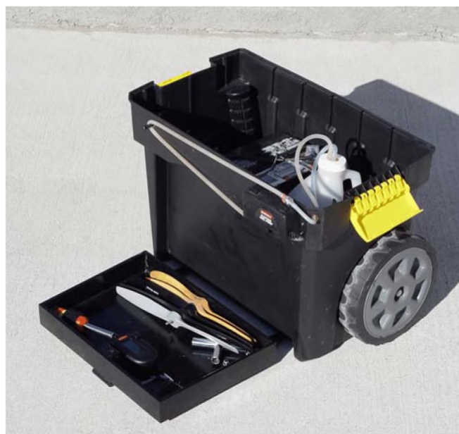
Photo 3: The lower section has wheels and the two clamps at the sides that lock the upper and lower sections together. The fold-down compartment is something I added (see text). Note the shortened fuel bottle (see text for details).
