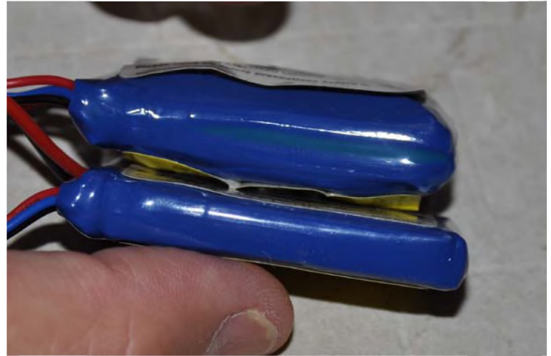
Photo 3: The failed pack is on top, and the good replacement pack is on the bottom.
