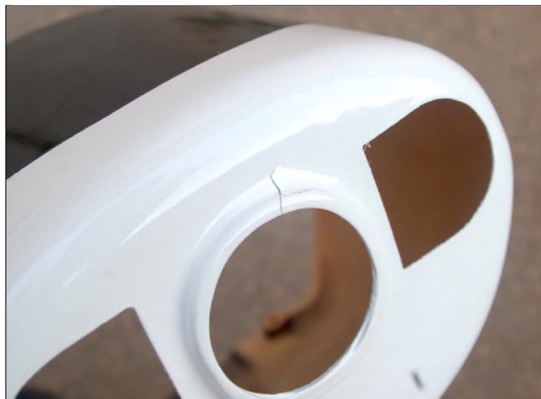
Photo 1: The fiberglass cowling comes nicely trimmed and painted. Mine showed evidence of mishandling via a few cracks.
