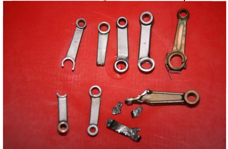
Photo 1 A very common example of 'evident mechanical problems' I see very often on my work bench. If the rod is broken the engine ceases to operate
