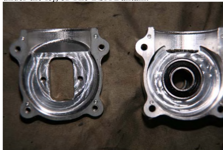
Photo 4-Intensive CNC work inside a quality crankcase so the parts that fit in are virtually shoe horned in to fit.
