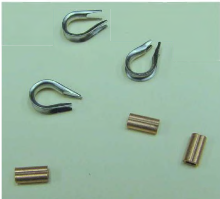
Photo 7: Wire thimbles and compression sleeves, used to attach braided wires
