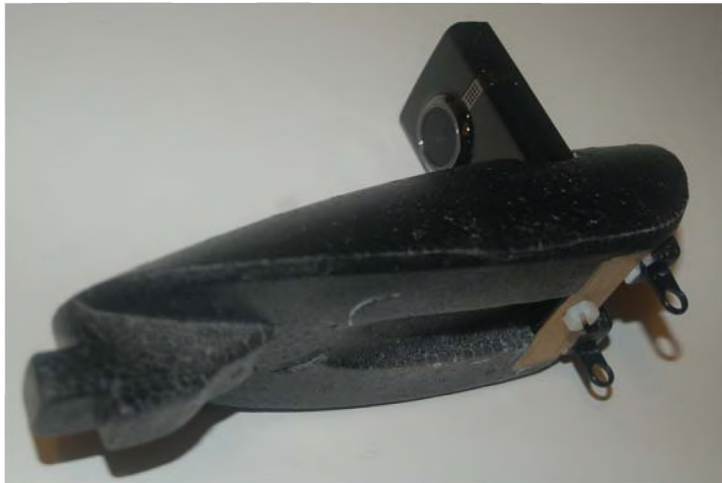
Photo 2: The stock foam canopy of the Multiplex Easy Glider was carved out to accept my Flip Mino HD camera. Not the lite-ply brace and a ¼-20 nylon bolt on the bottom.
