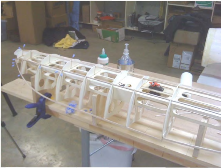
Photo 6: This photo shows Robert installing the stringers to the formers of the center line float of his Rufe. Notice the installed servo to control the water rudder.
