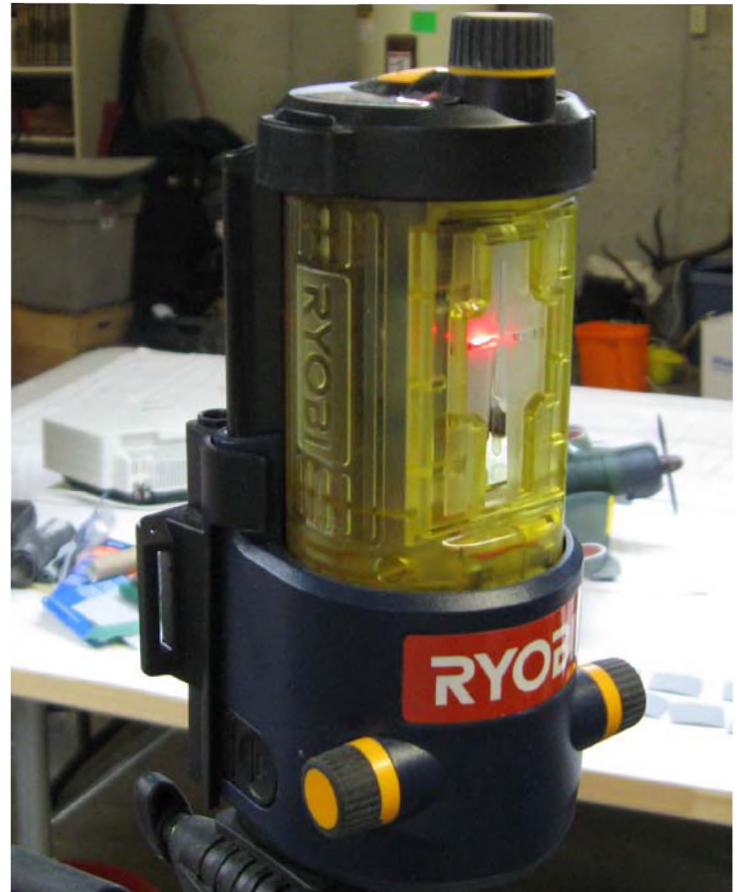
Photo 5: Robert purchased this Ryobi laser unit at a local hardware store for around $50.00. It projects both vertical and horizontal lines to be used in the alignment of various parts of the aircraft.
