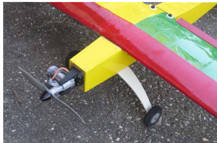
Photo 4: Patches front end, showing the SK 50 engine and the DuBro nylon & glass gear.
