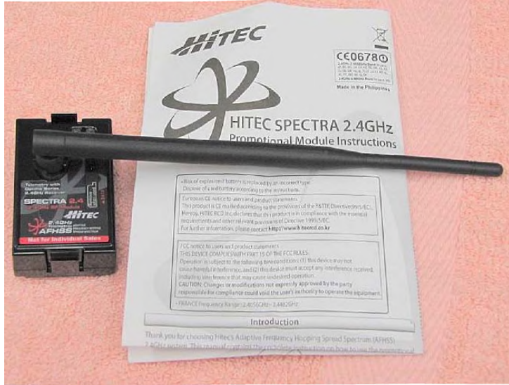
Photo 4: Hitec Spectra 2.4P transmitter module with attached antenna
