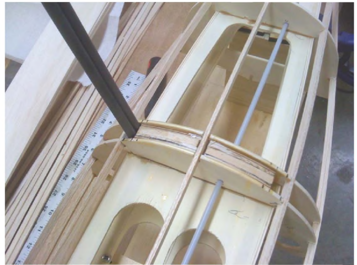
Photo 7: Robert designed the rear V strut mounting point on the center float to be both strong and light. He used a sandwich of balsa and ply. The strut is made of two carbon fiber rods.
