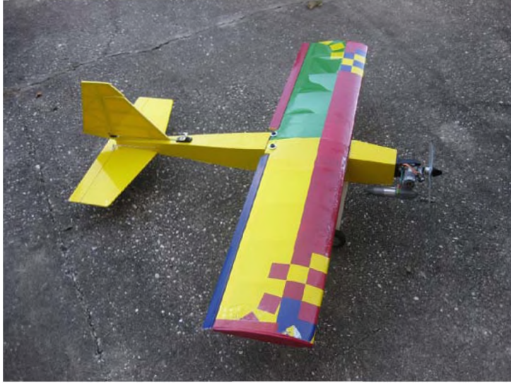
Photo 5: Patches side view. More clear tape patching a hole out near the right wing tip.
