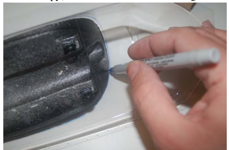
Photo 3: To use the Park Flyer Plastics canopy upgrade kit for the Easy Glider, you first have to trace the outline of the stock canopy on the clear plastic.
