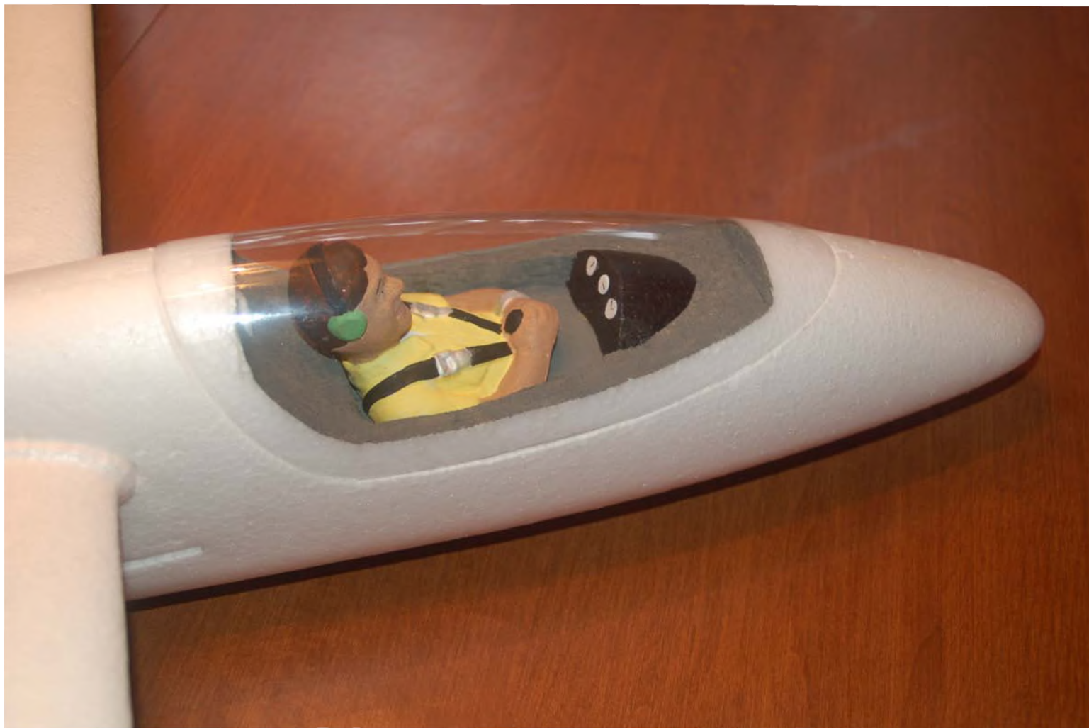
Photo 7: Although it's very simple, the canopy kit really dresses up the otherwise foam finish of the Easy Glider and gives it a bit of personality.
