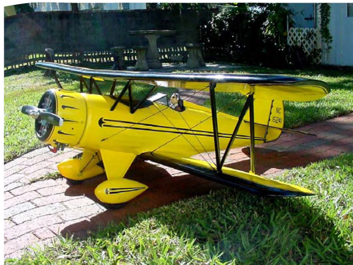
Photo 2: Fuselage covered with Koverall and Nitrate Dope.
