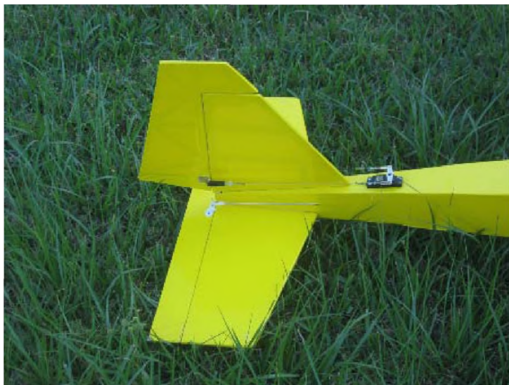
Photo 3: Patches' tail. Note pull-pull rudder servo. There is another servo underneath for the tail wheel steering.
