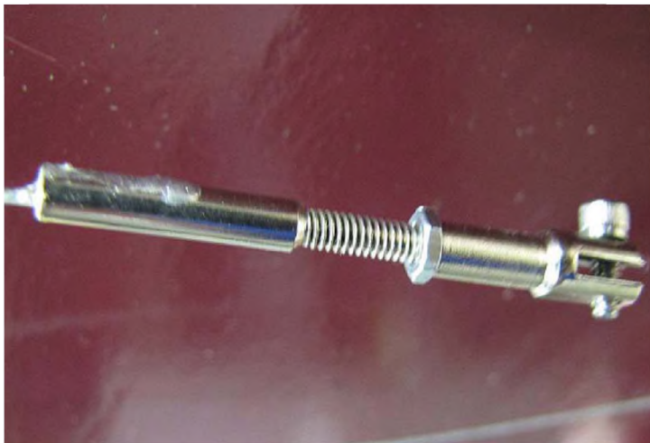
Photo 9: Be sure to leave threads for tightening rigging wires
