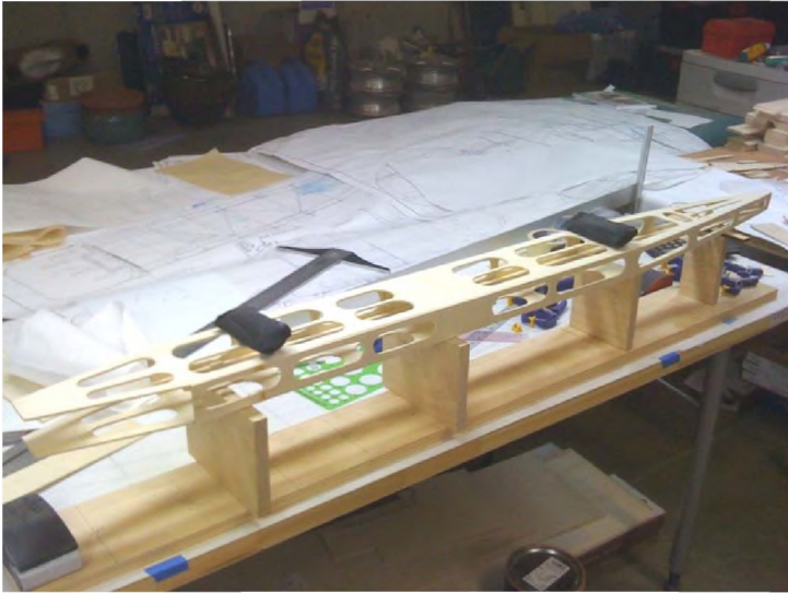
Photo 3: This is the main box beam Robert designed to support all the weight of the center line float. It runs the entire length of the float.
