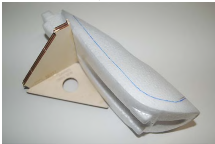
Photo 4: To prepare the stock canopy for cutting, I tack-glued scraps of lite ply to keep it square to the blade of my band saw. I cut along the blue line and used the bottom section as the foundation for the upgrade kit.
