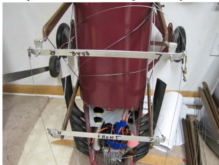
Photo 8: Wing center section joiner brackets to attach rigging wires
