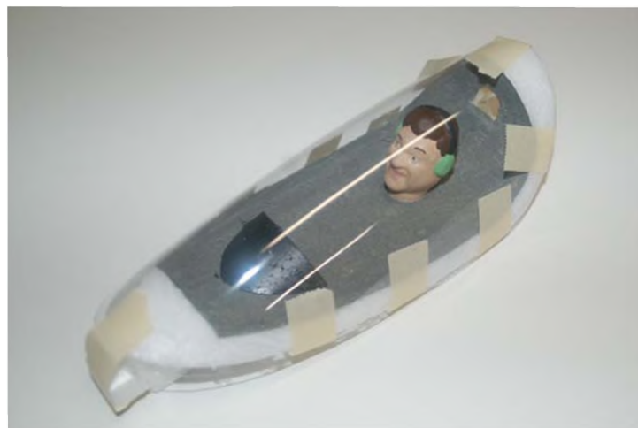
Photo 5: Drafter's tape holds the canopy in place while the glue dries. I didn't like the look of having only a pilot's head, so I removed the canopy and added a torso.
