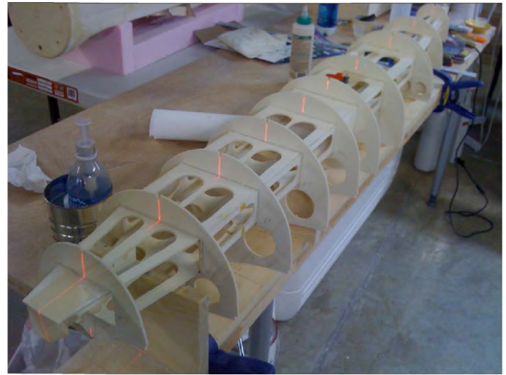
Photo 4: This photo depicts the center float box beam with formers installed, using builder's laser to align each former vertically.
