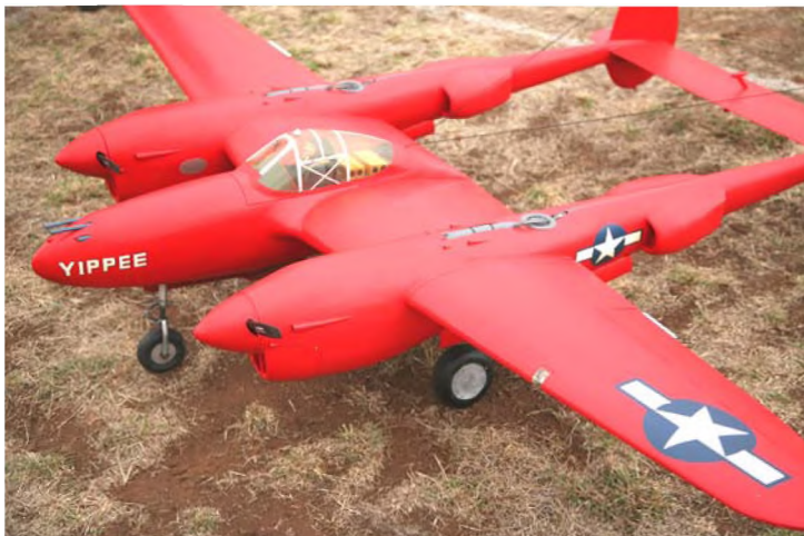
Photo 5: No scale detail missing, and lots of parasitic drag. At this angle, a motor cut would be fatal to the model.
