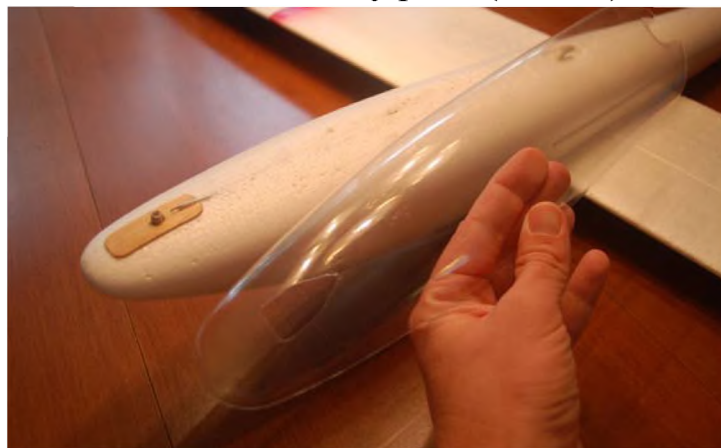
Photo 6: Drafter's tape holds the canopy in place while the glue dries. I didn't like the look of having only a pilot's head, so I removed the canopy and added a torso.
