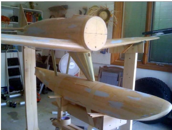
Photo 1: Showing attachment points for the center float. Notice use of fiberglass skin for main pylon.
