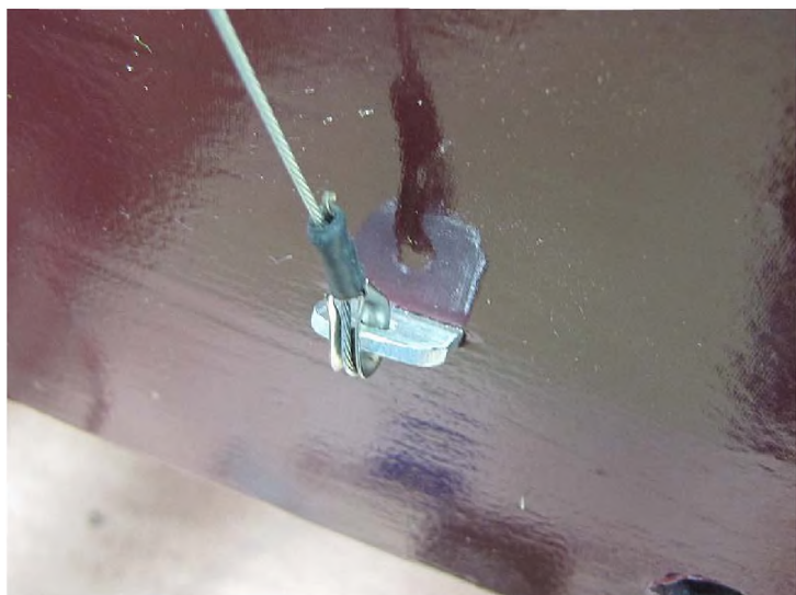
Photo 6: Metal fittings in fuselage for installation of flying and landing wires
