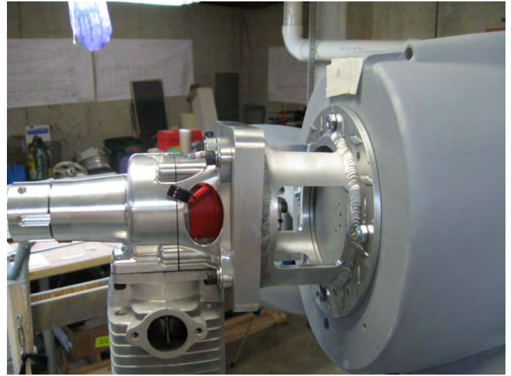
Photo 2: Robert's custom made aluminum engine mount; strong but light weight.
