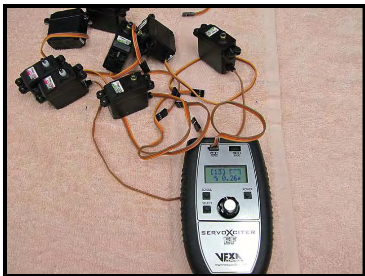
Photo 4: Vexa Servo-X-Citer used to test servos.
