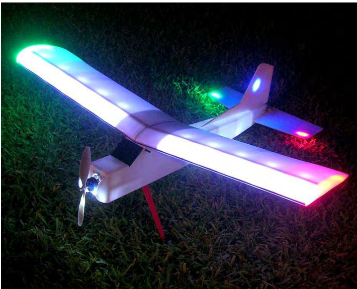
Photo 1: Lee Ray's "BEST Special" is a homebrew night-flyer design that illustrates good usage of internal LEDs for lighting.
