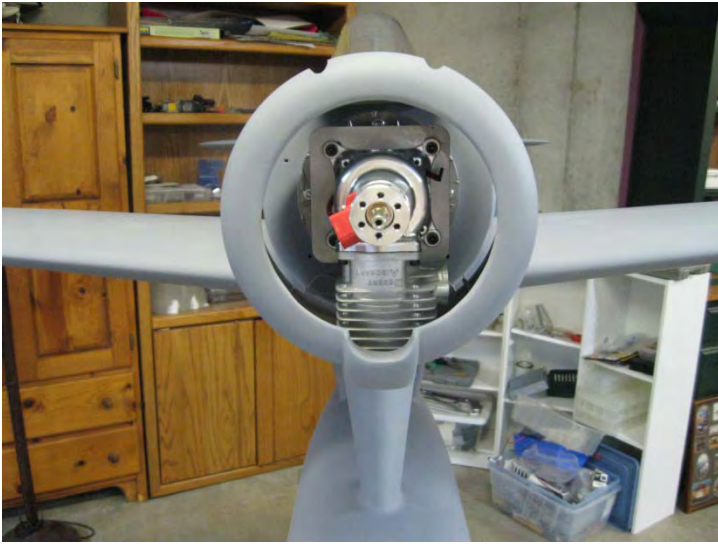
Photo 4: Front view of finished cowl, showing the cut channels of the fuse mounted machine guns that were fired over the top of the cowl.
