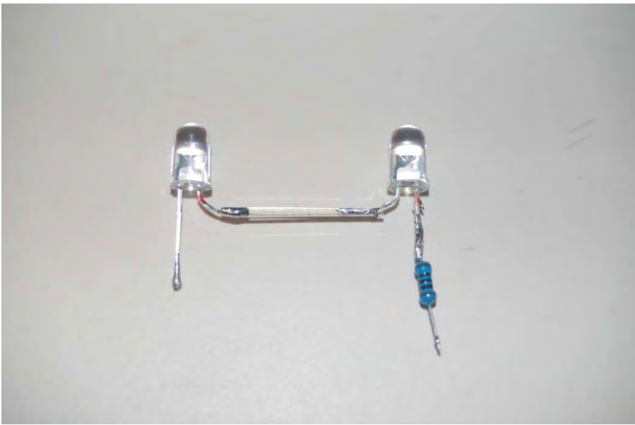
Photo 2: The two white LEDs in this photo were wired in series with a 100-ohm resistor to accommodate an 8.4-volt power source. The lower forward voltage of red LEDs means that three lights and a 100-ohm resistor can be hooked to an 8.4 volt source.
