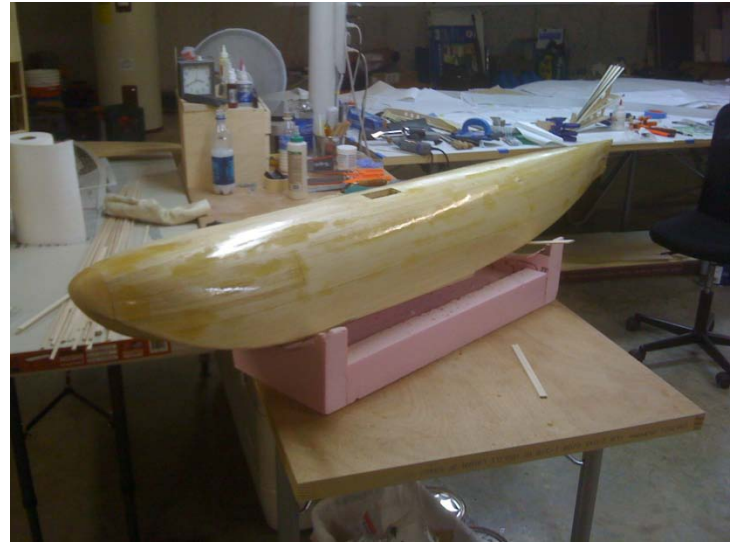
Photo 6: Main float after being fiber glassed with 3/4 oz. cloth and Zpoxy resin.
