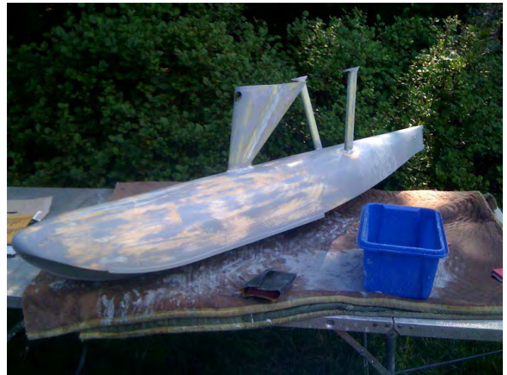
Photo 7: Main float showing the on going process of priming, sanding, filling, and then re-priming to get a truly smooth finish.
