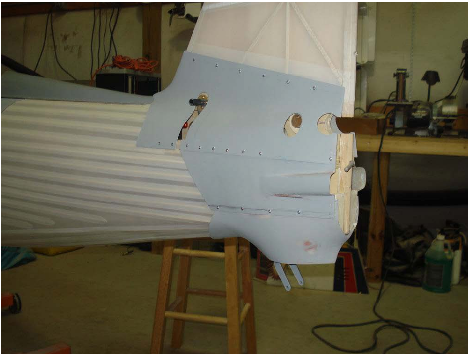
Photo 2: Lonnie Johnson's third scale fuselage showing the fiberglass fairings.
