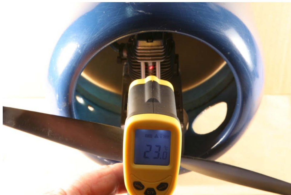
Photo 7: Pin pointing the area of the engine inside a cowl. You can gain a lot of valuable information carrying out this type of test.
