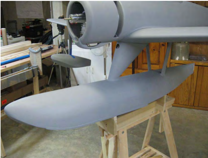
Photo 5: Finished bottom of cowl showing cut out in the lower scoop to accommodate the engine head. Note the cowl flap opening in rear for cooling and scale appearance. The flaps will be installed before final paint. Also notice the reinforced main float chine areas along the bottom of the float.
