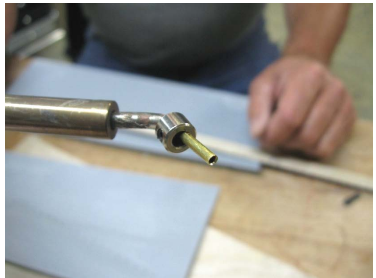
Photo 9: Homemade flush rivet making tool consisting of variable heat soldering iron, brass tubing to match the needed diameter of the rivets, and wheel collar to clamp the brass to the heating tip.
