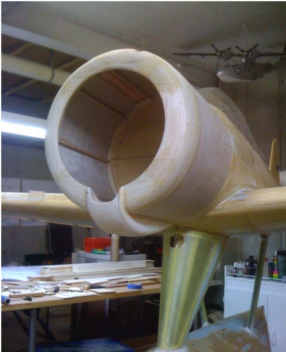
Photo 3: Custom built cowing using light ply and balsa. Notice the internal light frame and Spruce in upper cowl for the gun channels cut out areas.
