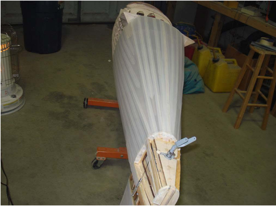
Photo 1: Lonnie Johnson's third scale fuselage showing the reinforcing tapes over the stringers.
