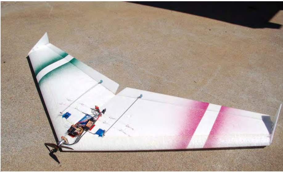
Photo 6: By omitting the covering and using a small, modern power system, my Zagi night flyer weighs less than half what it did 10 years ago. It will fly SLOWLY.
