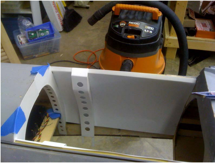
Photo 4: The start of making the left side of Robert's A6M2-N Rufe's cockpit. Made from sheet styrene plastic purchased at a local hobby shop. Robert used photos of the actual cockpit of an A6m2 to make it as close to scale as he could make it.
