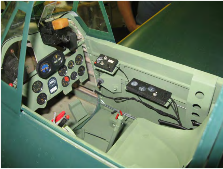
Photo 8: Notice simulated hydraulic lines made from plastic rods. Also the gun actuator on the throttle handle. One machine gun has been installed. Notice the manual cocking arm on the right side of the gun
