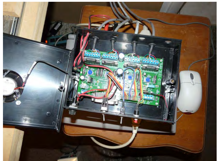
Photo 3: Finished driver board assembly mounted in plastic project box (not included in driver kit).
