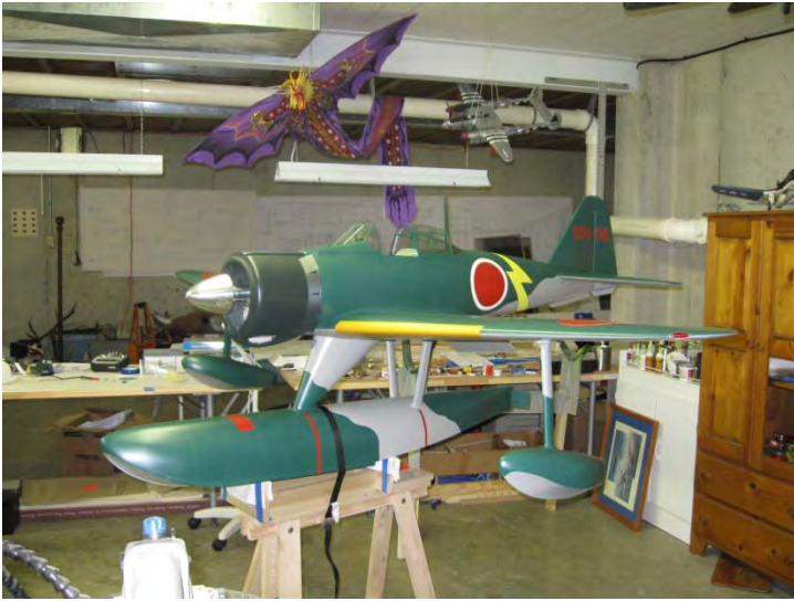
Photo 10: Left view of the Zero after paint work is finished. Note cowl flaps installed and tiny nav lens on wing tip.
