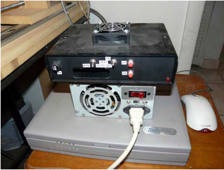
Photo 4: Completed driver board assembly mounted to power supply from an old computer. Note switch on power supply and fan on driver box.
