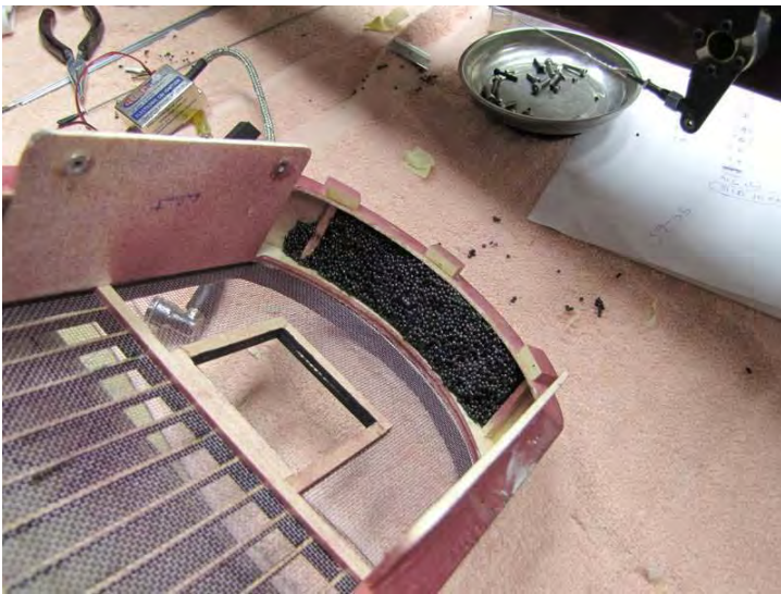
Photo 7: Lead shot and epoxy can be added to a short wooden cowl, but not longer plastic or glass ones
