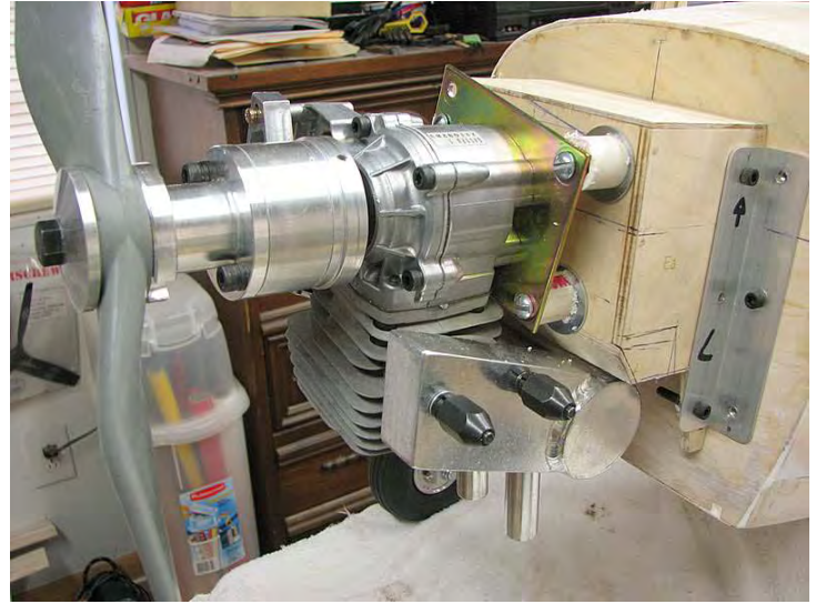
Photo 8: If a small plywood box is added on top of this engine mount, lead can be added
