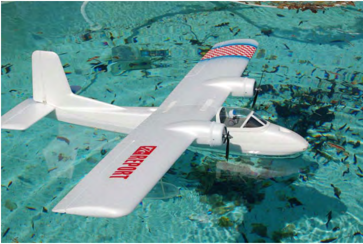
Photo 3: My Twinstar II seaplane conversion floats comfortably in Bill's pool. The clear plastic hull and tip floats are difficult to see now, but they'll soon get a coat of paint. Note the broken starboard prop...oops.
