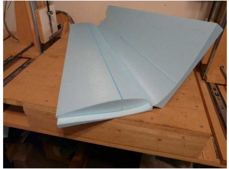
Photo 5: Finished wing half with spar slots
