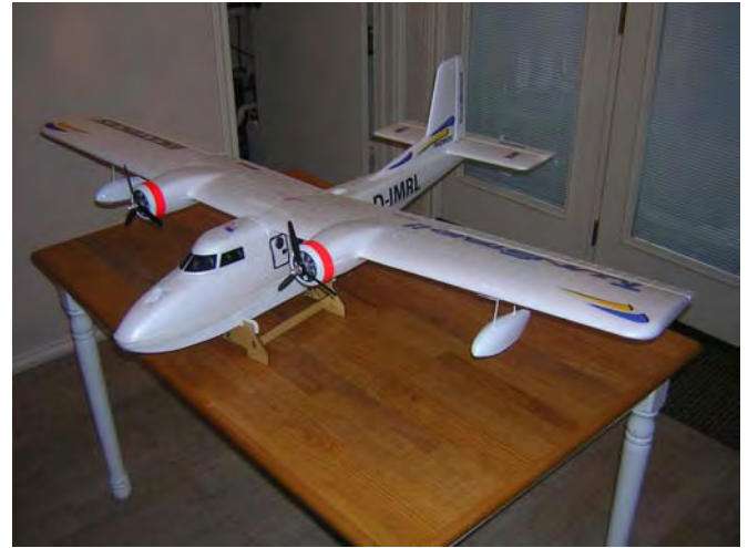
Photo 4: Elwood Kotil's Twinstar uses counter-rotating, 3-bladed props. He finished the conversion quickly and maidenied it from his backyard lake (Kotil photo).
