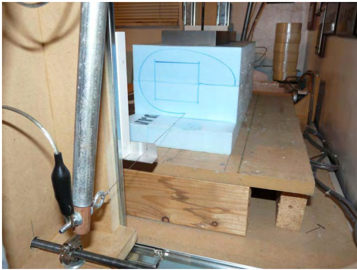
Photo 7: Fuselage section being cut. Note hotwire resting in aluminum slot on Y axis tower.
