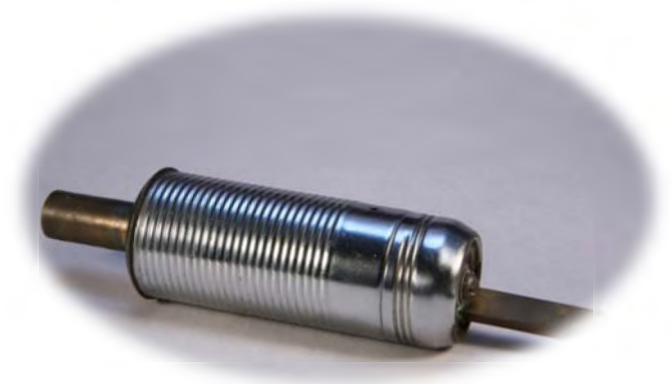
Photo 1: I made this .40 size muffler from a torch body to connect with a curved header.
