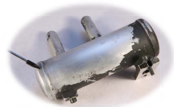
Photo 4: A well used muffler with nitro attack on the paint. Note the return indicated on the end cap.
