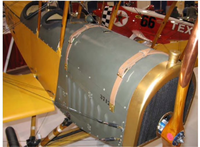
Photo 3: Fine detail of the Curtis Jenny including the leather cowl straps and the copper plating of the leading edge of the prop
