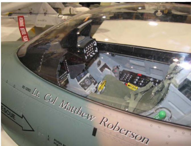
Photo 22: Close up of Graeme's F-16 cockpit. Even the panels light up. Notice the ejection seat pull handles, and seat padding with belts.
