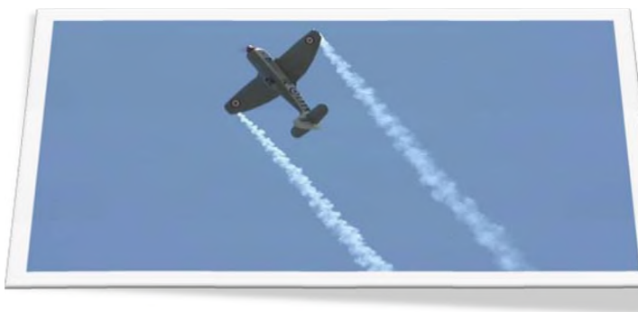
Photo 27: Notice the wing tip smoke system. They are really small smoke bombs.
