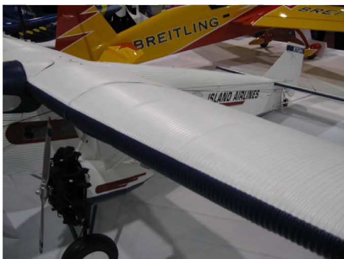
Photo 18: Detail shot of the Tri-motors corrugated skin along with all the control surface cables present on the external fuselage sides.
