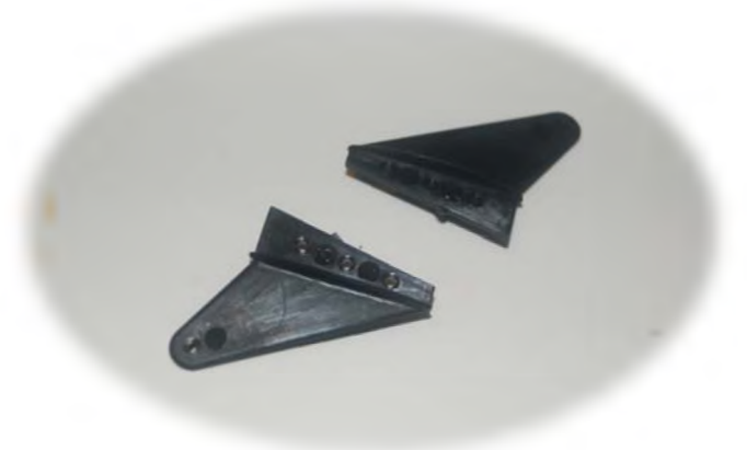
Photo 4: HDI Products also sells these molded control horns that glue into place. I'll be trying them on an upcoming project.
