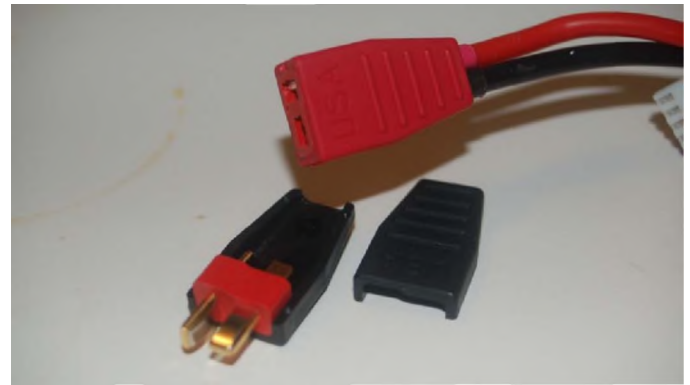
Photo 3: These glue-on shrouds from HDI Products provide a large, textured surface that makes it easier to disconnect Ultra Plugs.
