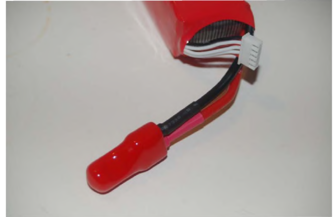
Photo 5: Battery Buddies provide insulation to the exposed ends of Deans Ultra Plugs. They can also be used to identify the charge state of a battery.
