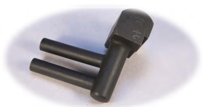
Photo 5: Double expansion chamber for a tight installation. The top section (manifold) was machined from bar stock - drilled hollow and the open end plugged and brazed.
