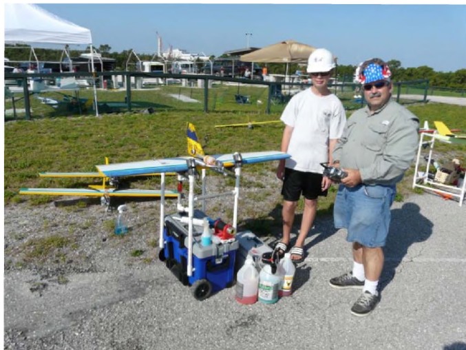
Photo 10: Flight stand on rolling tool box by Craig Buttery
