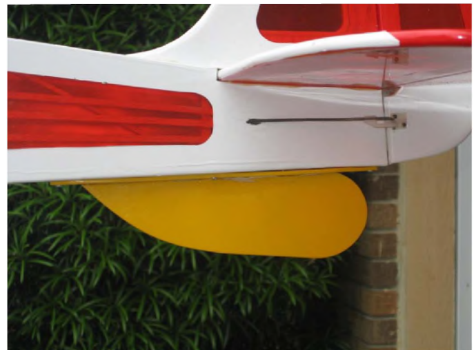
Photo 5: Sub fin included in the Great Planes ARF Fiberglass Float kit.
