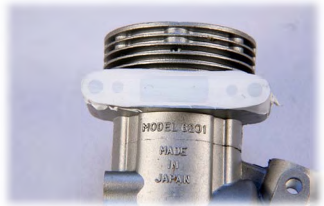
Photo 6: Pull the tape over the manifold and tear it off. Two or three layers will do a good job.
