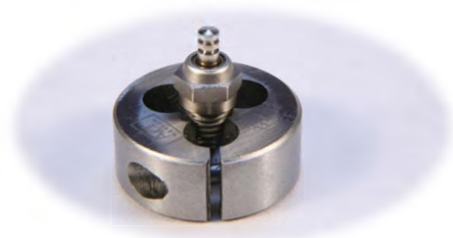
Photo 1: This is an adjustable die that I have set for the best fit for a glow plug.
