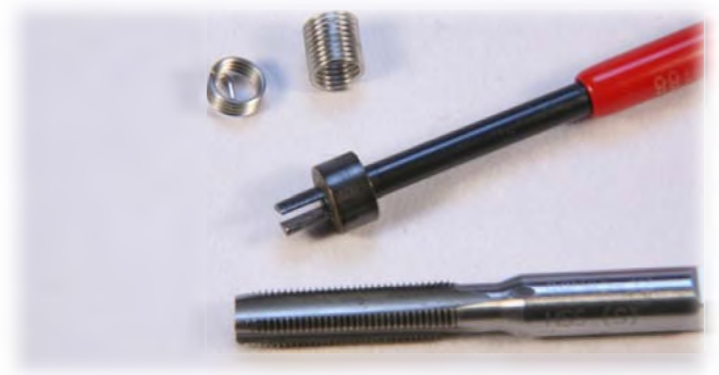
Photo 2: Thread coil fitting tool, special thread tap and the stainless steel, diamond section, wire thread coils.
