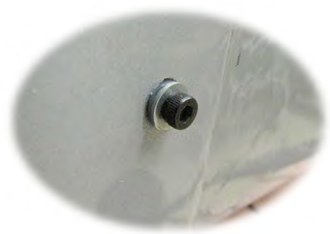
Photo 12: Mounting bolt tightened and tubing mushrooms out to form a vibration isolator.
