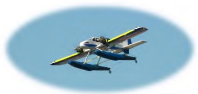
Photo 8: Our TwinStar on floats. During the time I had it, it was necessary to recover the wing. I used fluorescent yellow Ultracote for visibility and installed larger ailerons. The struts are U-Can-Do-3D landing gear ordered from Tower. The floats are balsa sheeted foam with lightweight fiberglass cloth applied with water based polyurethane and then sprayed with blue Lustrekote.
