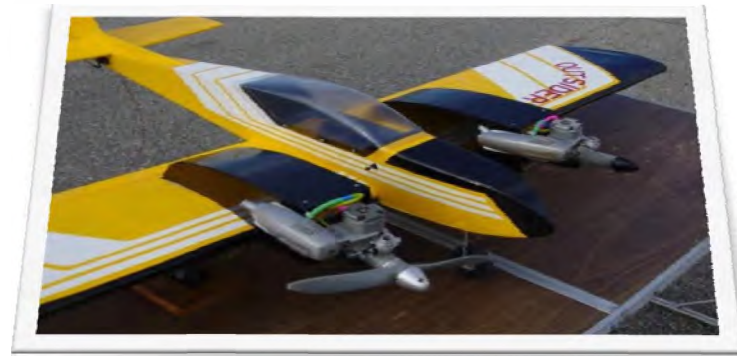
Photo 2: The Outsider, a modified Goldberg Tiger 2 ARF by "Flaps" Laffert with two OS .46AX engines. Each engine has 8 degrees out thrust to counter yaw if one engine or the other fail in flight.
