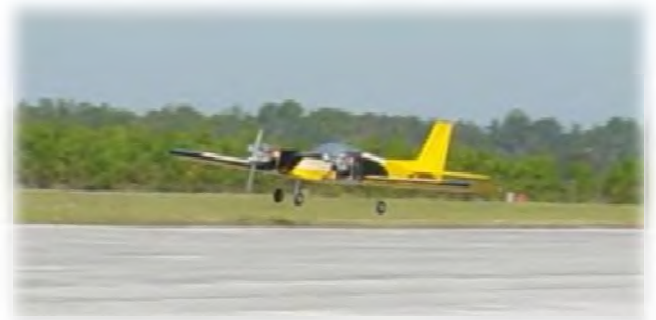
Photo 3: Ed brings the Outsider in for a landing on one engine during the "prove that out thrust will work" engine out testing. Notice: No rudder is being used.
