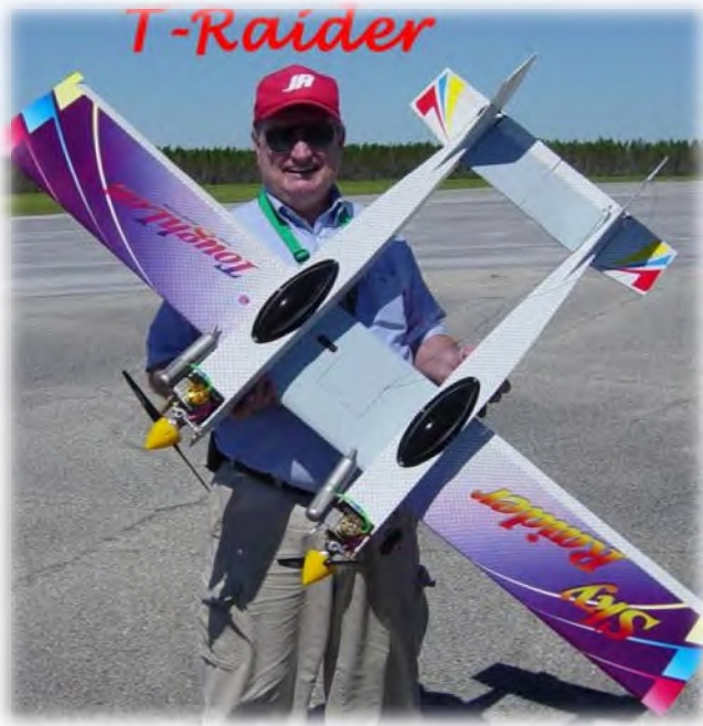
Photo 4: Ed and his T-Raider, a twin fuselage airplane build from two Sky Raider Mach II ARFs. The power is two GMS .47 engines with some out thrust, but not 8 degrees. The GMS .47s were later replaced with two OS .46AXs. The T-Raider was an excellent flying plane, probably my best flying, sport/aerobatic twin.
