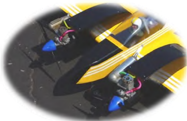
Photo 6: The Outsider with two different size, unmatched engines. On the left nacelle is a Thunder Tiger .46Pro with a Tower muffler for a little extra rpm and an 11-6 prop. On the right side is Flaps' well run, plain bearing Thunder Tiger .42GP with the stock muffler and a 10-6 prop.
