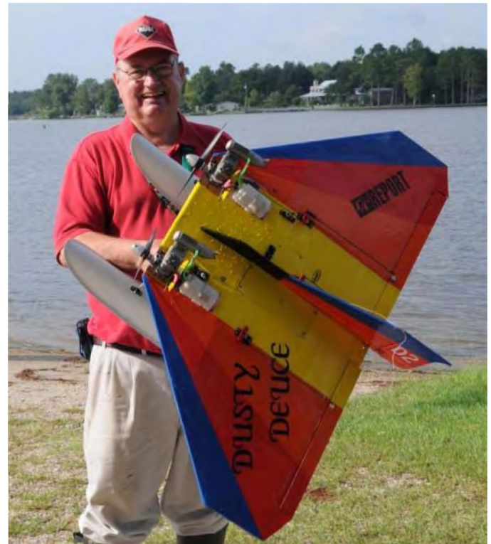
Photo 9: Ed and his Sea Delta, a twin engine, delta wing, seaplane. It was built by Flaps Laffert. The power is two OS .46LA's. Fiberglass floats that were given to me.
