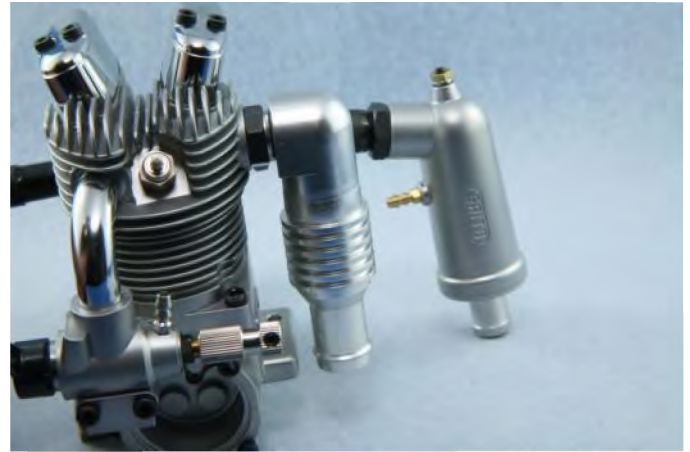
Photo 3: Compare the total width with the TurboHeader and the supplied standard muffler.
