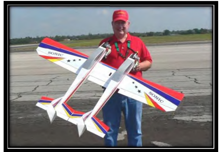
Photo 5: Ed showing his Double Sonic which was built from two Sonic 25 ARF kits. Wider ailerons and rudder were also installed. The power was two OS .46LAs. The Double Sonic was a good flying twin, but not as good as the T-Raider.
