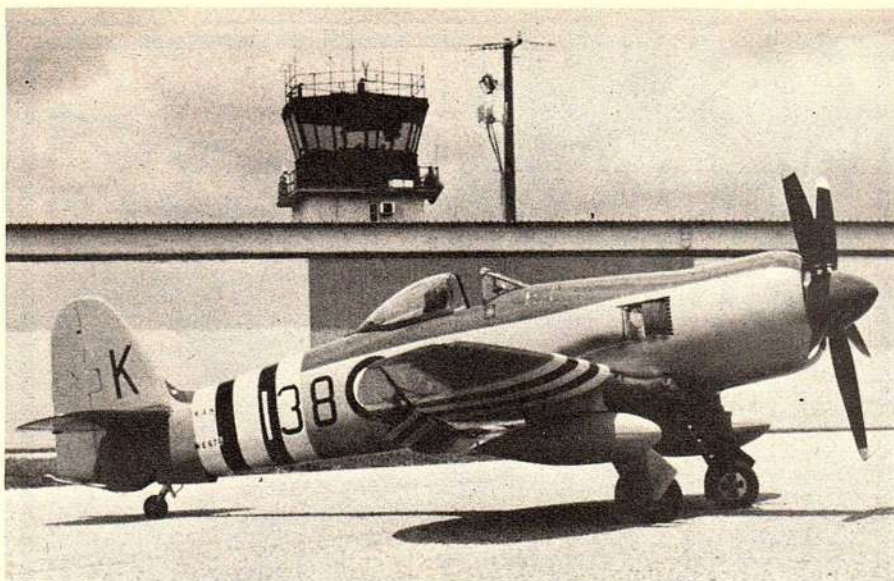
Vito Tomeo's Sea Fury uses a gear drive to achieve scale speeds. Feature article on this model appeared in the December '80 issue.
