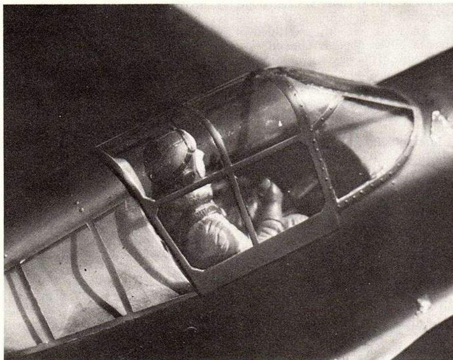
Modifying the cockpit is a piece of cake, with the rear windows replaced by clear butyrate.
