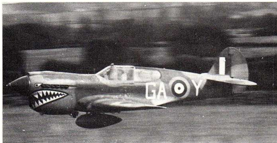
The P-40 is a big machine, with a 65" span, and it flies nicely on an over-propped .60 engine.
