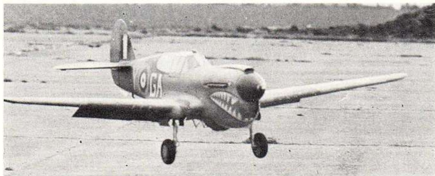
With those big split flaps lowered, the Kittyhawk drags in for a slow landing.
