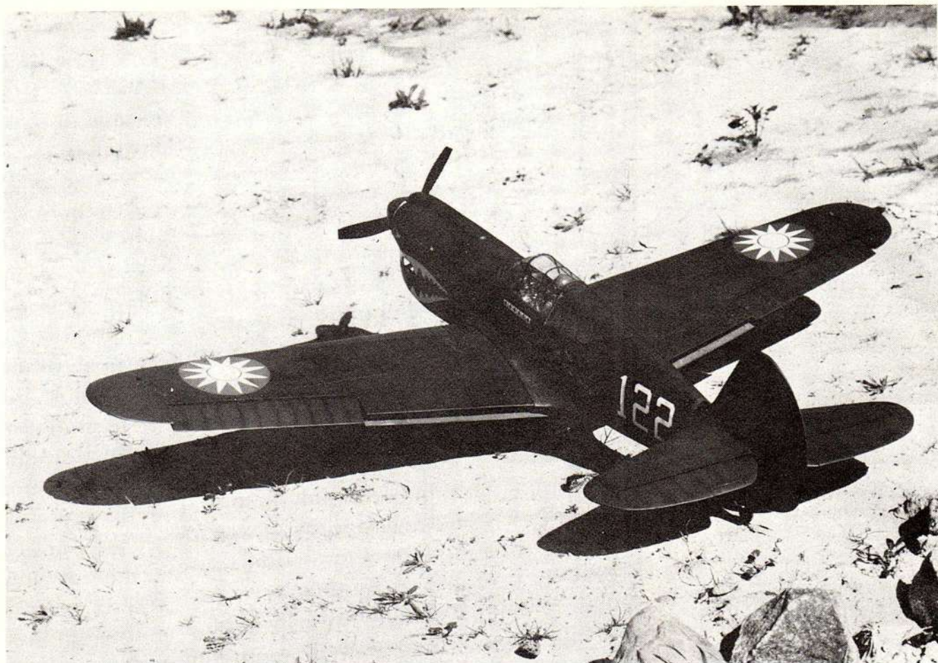
Plenty of wing area and a comfortable amount of dihedral (plus some washout) make the P-40 a very stable machine.
