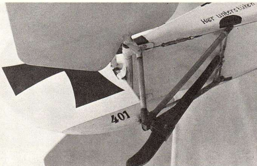
The tail skid also serves as the bottom hinge for the comma-shaped rudder. Shock absorbing via a rubber band.
