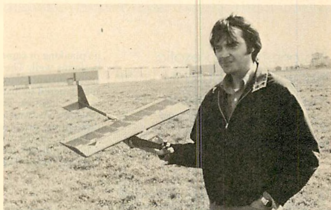
This is Bob Aberle's Nothin' Special (an FM design) with a "V" tail removed and conventional tail feathers substituted. Bob explores all possibilities. At left: Bob again in the field, original "V" tail seen on Nothin' Special. It was featured in May, 1975 FM issue. It will meet new rules as shown but a cowled engine would reduce drag. Below: Chuck Silver and his original ship Disaster. He would need a canopy to meet a 4" minimum fuselage height rule.
