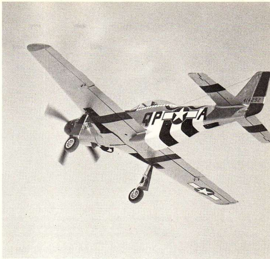
Sorry this shot had to be gear down, but we couldn't get the gear to cycle. Note that tailwheel is jammed inside the well, because we lost the centering spring on the Rhom unit. Landing was so slow that only a sliver of paint was scratched from the rudder.
