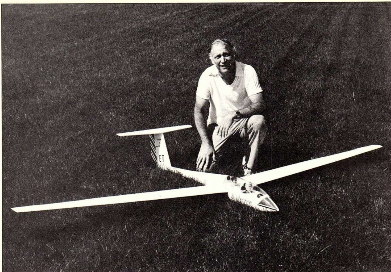
Eugene Bornoski's Twin Astir is an original design. The 120" span model weighs only 5½ pounds. (Hiner photo)
