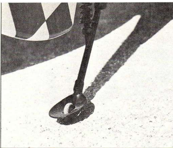
John installed a small wheel in the "spoon" of the scale tailskid, to facilitate ground steering on paved runways.
