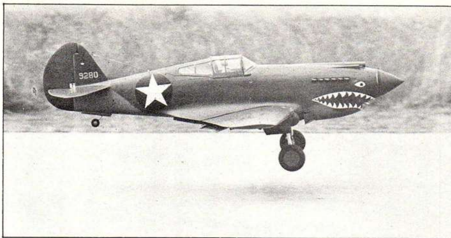
Well deserved winner in Giant Scale was this scratchbuilt P-40 by Col. Art Johnson. An O.S. .90 powers this 15-pound model.
