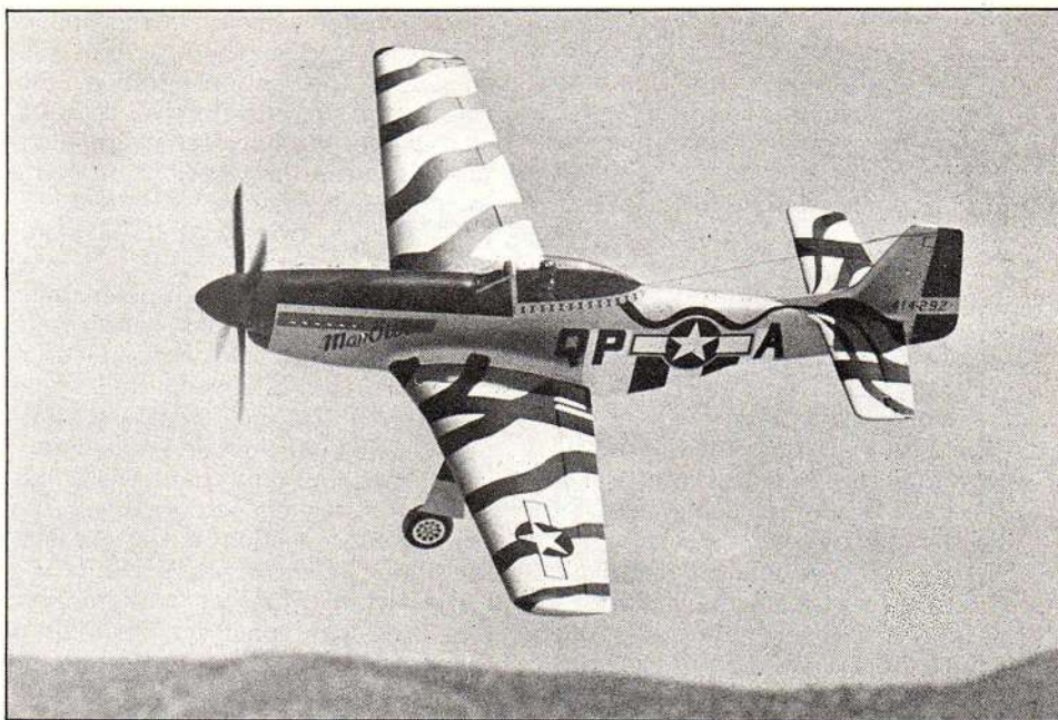
The intricate O.D. striped paint scheme was done by the trained hand of Rick Lewis, a virtuoso with an airbrush. Paint is all automotive lacquers, to minimize weight.
