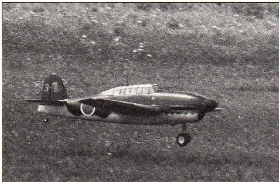
Ignominiously coming in with one gear hung up, the Judy prepares to land. Because of its low airspeed, the airframe suffered no damage.
