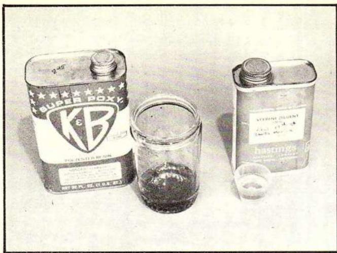
Mix three ounces of styrene monomer to eight ounces of polyester surfacing resin. Do not add hardener to this batch.
