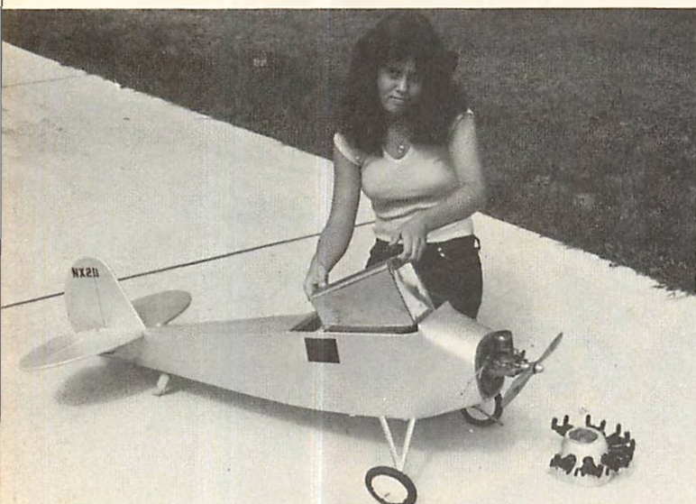
The R/C is all but lost within the cavernous interior, Cables to the rudder and elevator work well. Radio should be full forward if a large tank is ever contemplated. Left: Nancy McGovern shows how a standard gallon tank fits.
