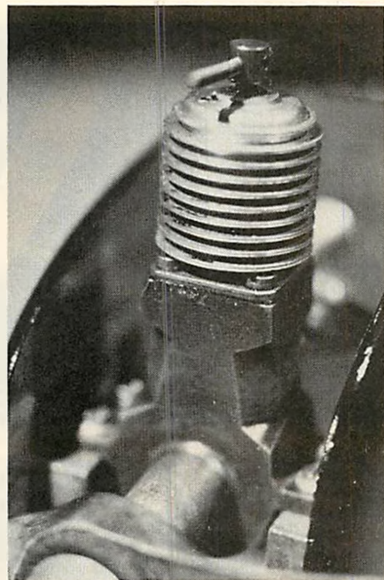
The famous English Mills 1.3cc (.09c.i.) (above) mounted in a reconstructed old timer free flight. Three currently available diesels (left). Top, the ball-bearing D.C. Rapier that comes complete with silencing manifold. Lower left, the D.C. Dart, a .5cc (about .03 c.i.) diesel that is a big favorite with F/F scale builders and lower right, the Webra Record, an .09.
