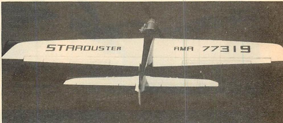
The Starduster is a very clean airplane with its thin fuselage profile and jet-like appearance. With no canopy on the ship, the looks are improved by simply painting one on. No points for detail in stunt.
