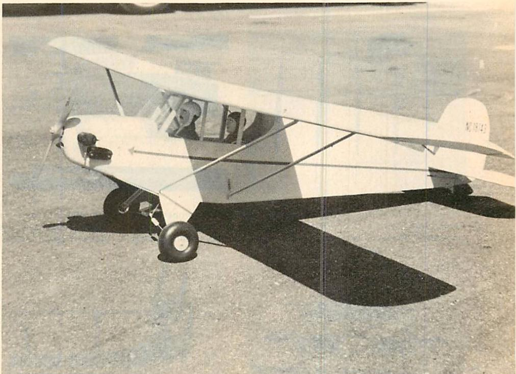
An ancient Super Tigre .51 still puts out more than enough horsepower. Uses a 3/4" K&B extension shaft. Cowling is from a Sig J-3 Cub. Tailwheel steering with horns is simple. At top: in flight, dead stick.
