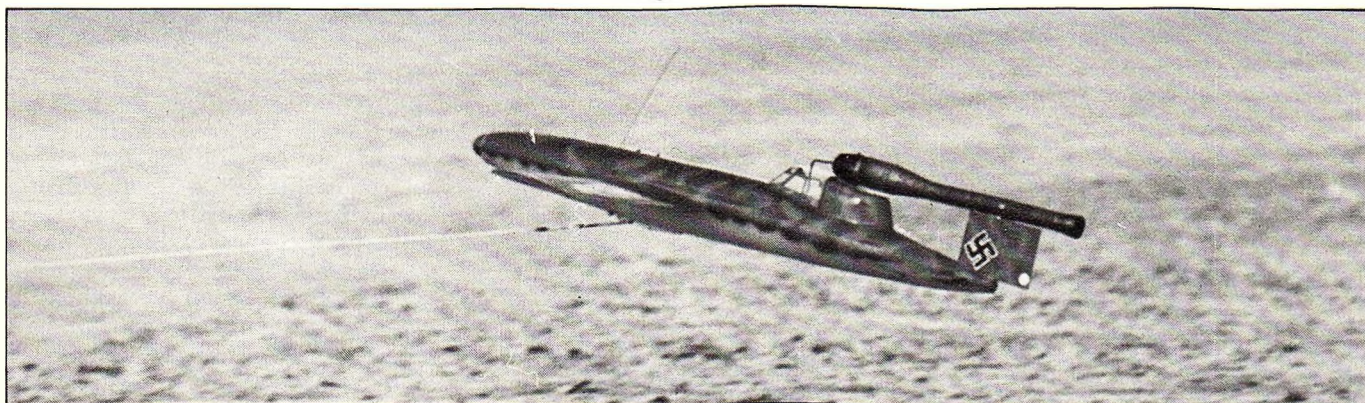
The pulse-jet powered Buzz Bomb, being catapulted off its elaborate launch ramp. The photo clearly shows the bungee cord which helps it get momentum. The jet reaches speeds in excess of 200 mph!
