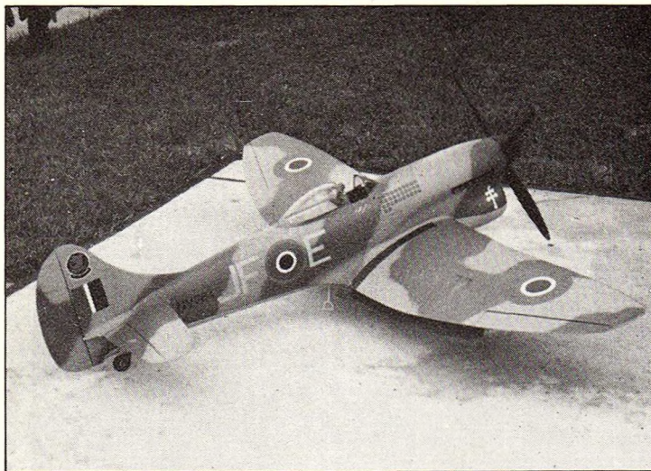
The elliptical wing is very efficient, which is why this 80" span fighter can fly on a straight-drive .90.
