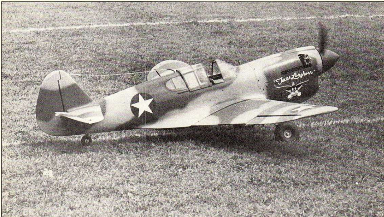
It may not look it, but this P-40 weighs 32 pounds, and has a 95" span. A Kawasaki 3.15 does the hauling.
