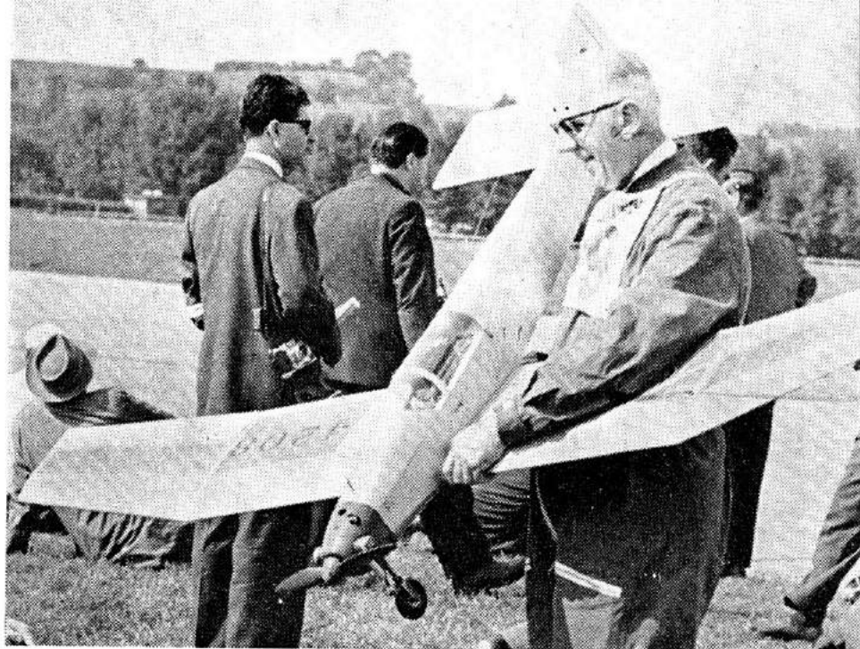
Dr. Gobeaux holds son Jean-Pierre's model. Nose wheel has pneumatic brake.
