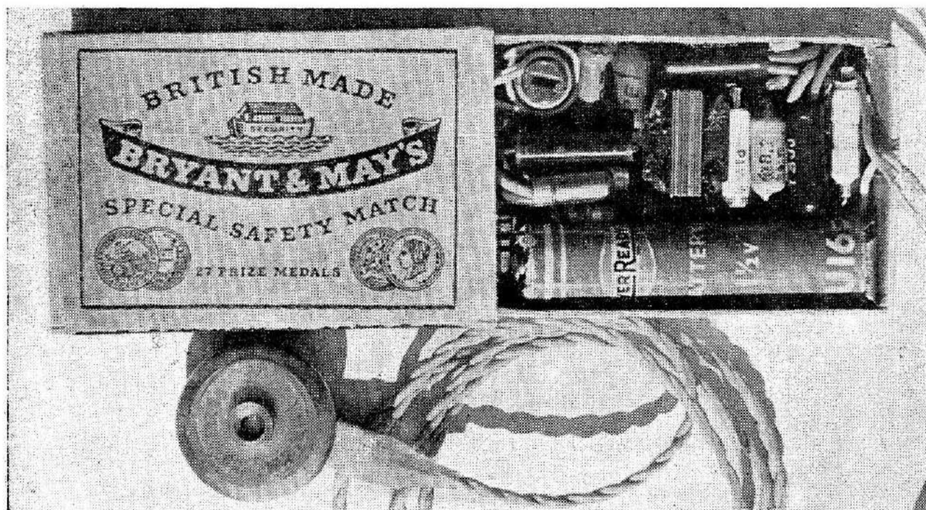
FIG. 1. Miniature receiver stowed in its matchbox. As the author dryly informed us replacement of case as necessary can be cheaply effected!
