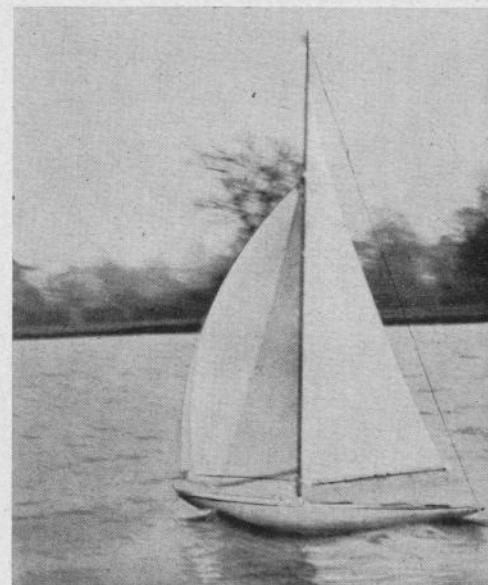
The author's successful A Class Yacht "Prelude" running with spinnaker. Note particularly the perfect wave formation. Sailing of this quality is to be expected of "Festive" which, by a process of evolution in design, carried out over several craft, will possess some of those characteristics usually only to be expected of larger yachts.
