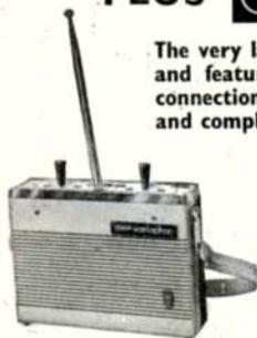
Crystal stabilised hand-held all-transistor transmitter with 50' chrome telescopic aerial.
