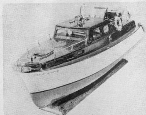
Section III. Freelance Cabin Cruiser built by E. G. Wilson of Winchmore Hill. All fittings handmade from brass. Power—Bassett Lowke electric motor. Hull 23½ ins. long, beam 6 ins., made from the solid. Photographed by L. C. Mason, as above.
