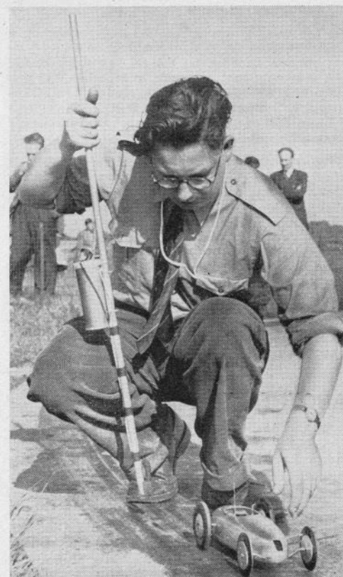
Top: The neat and easily transportable push-stick with bracket for a Nife battery, constructed by the author, and above: I. W. Moore of Derby with another type of stick, carrying a dry battery for Glow-plug heating.
