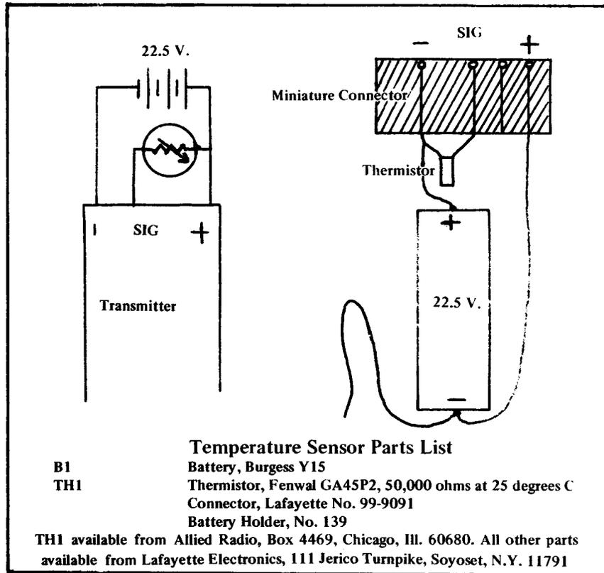
should be mounted so that the glass bead just barely sticks out of the body tube. The in-flight telemetered signal should be received on the ground and tape recorded. In addition, the rocket's altitude should be tracked and recorded frequently during the rocket's descent. The tracking observations and their relative times should be carefully recorded, as in Table 2.
