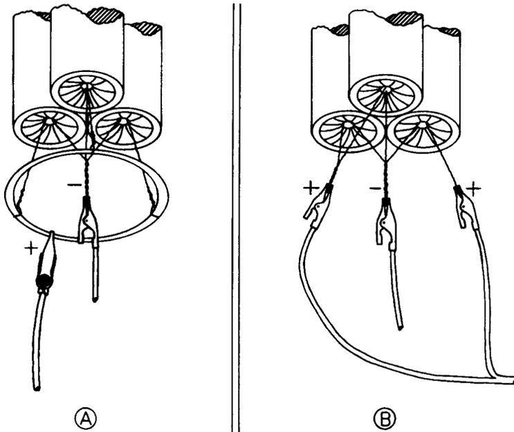
Figure 7. Two modern methods of parallel cluster ignition using nichrome or prefabricated ignitors. A: the Estes method, using a "bus ring" of metal for one common terminal. B: the Centuri method, using a "cluster clip-whip" to provide two clips of identical polarity. A similar multiple-clip arrangement is used by RDC.
