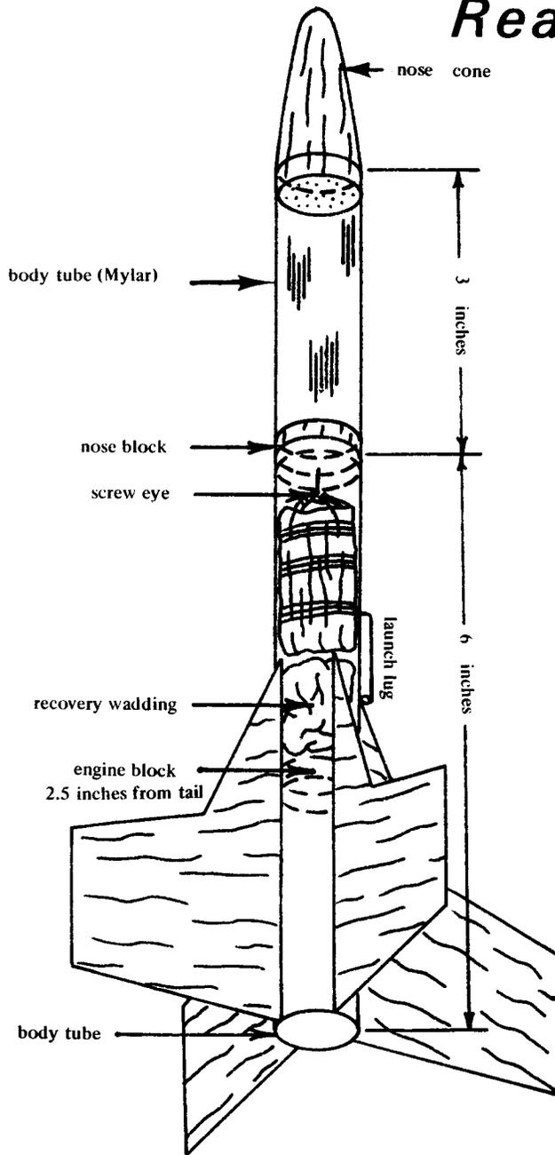
The *Lunar IV*, designed by Joseph Mann of Toronto, Ohio, is an extremely stable sport rocket due to its large fin area. It may be flown with any standard engine. Joe suggests that a booster may be added to the *Lunar IV*.
