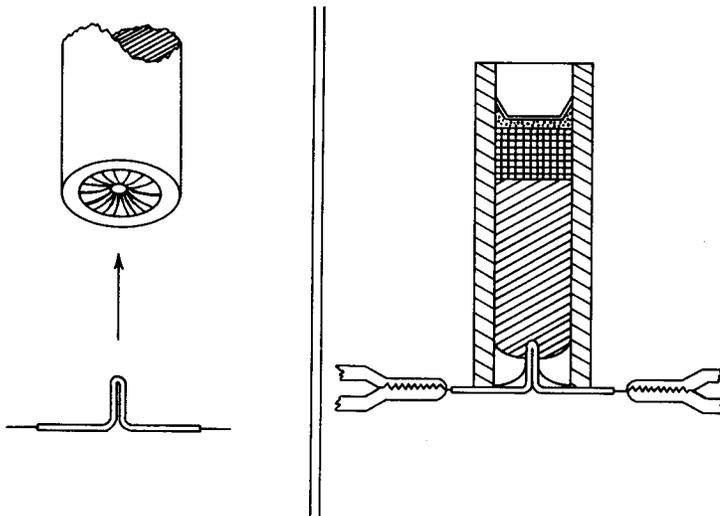
Figure 1. Electrical ignition using Jetex wick, 1957. Left: Jetex wick formed and stripped for use as an ignitor. Right: ignitor inserted into engine nozzle, bringing up against propellant grain, and gripped by Muller No. 85 alligator clips from firing circuit.
