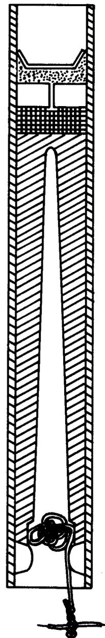
Figure 4. Ignition of Coaster "Super Jet" engine by Jetex wick, 1960. the "Starting ball" of wick has been inserted into the nozzle; its trailing strand extends down one side of the grain (to which it is taped) and is twisted together with the starting wick.
