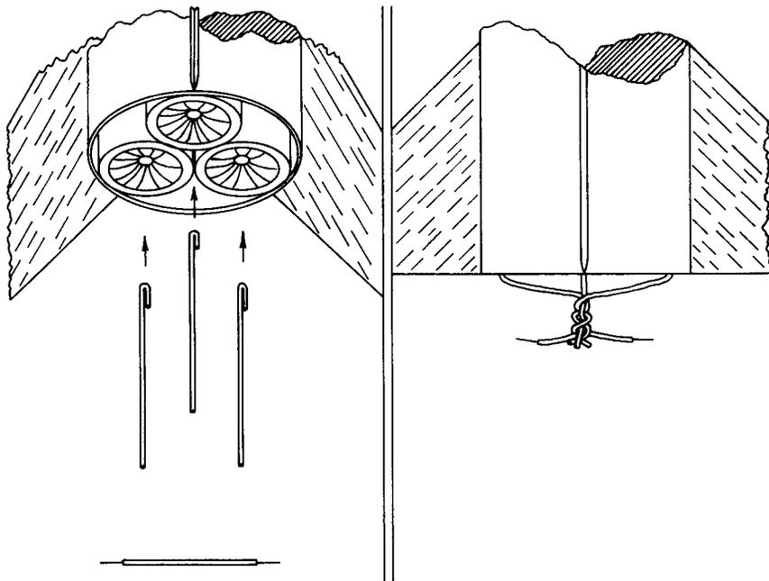
Figure 3. Cluster ignition using Jetex wick, 1959. Left: lengths of Jetex wick prepared for insertion into the engines of the cluster. Right: engine wicks have been inserted and twisted together with the starting wick to form electrical ignitor.
