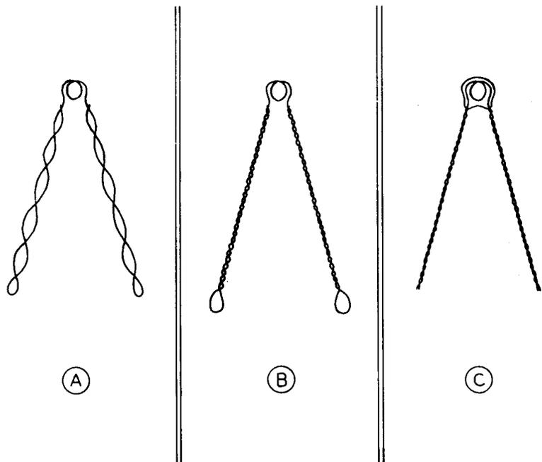
Figure 6. Nichrome ignitors developed by Marshall Wilder. A: loosely-doubled form used at NARAM-4, August, 1962. B: twisted-lead ignitor, early 1963. C: drill-twisted ignitor with lacquer coil coating, late 1963.
