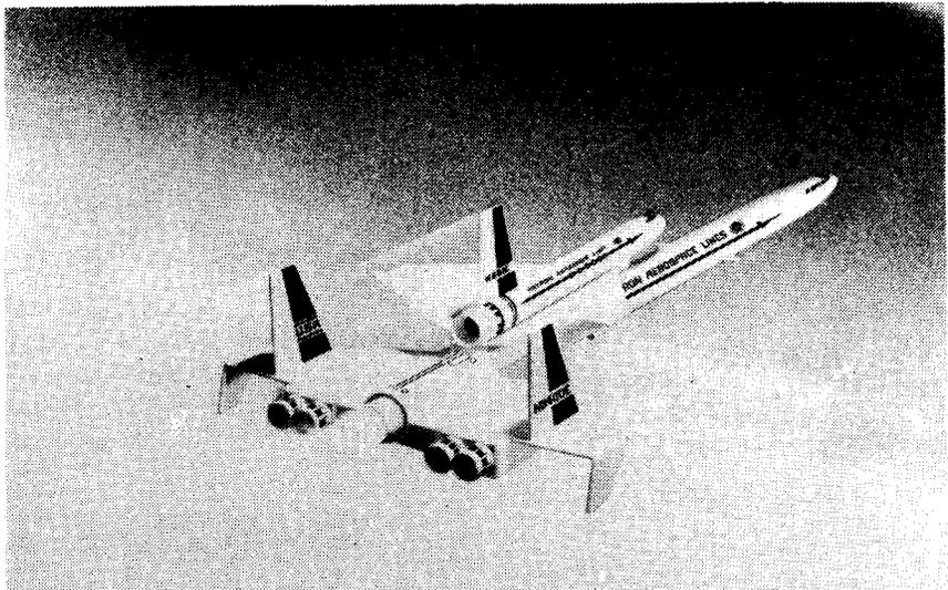
The **Orbital Transport**, a new concept in boost glider design, has been introduced by Estes Industries. The model is launched vertically with a single engine in the booster stage. After burnout, a small piggy-back glider separates from the main vehicle and glides back to earth. The booster is re-
