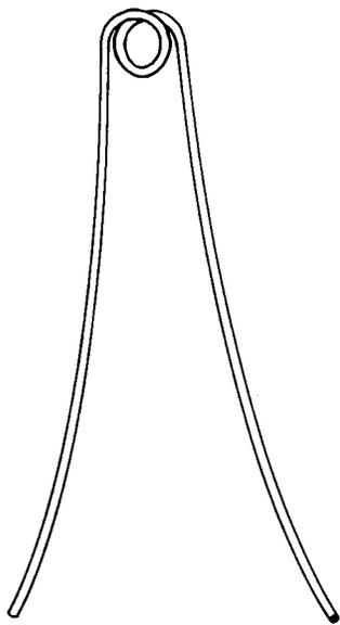
Figure 5. Nichrome ignitor, early 1962, showing detail of the heating coil.
