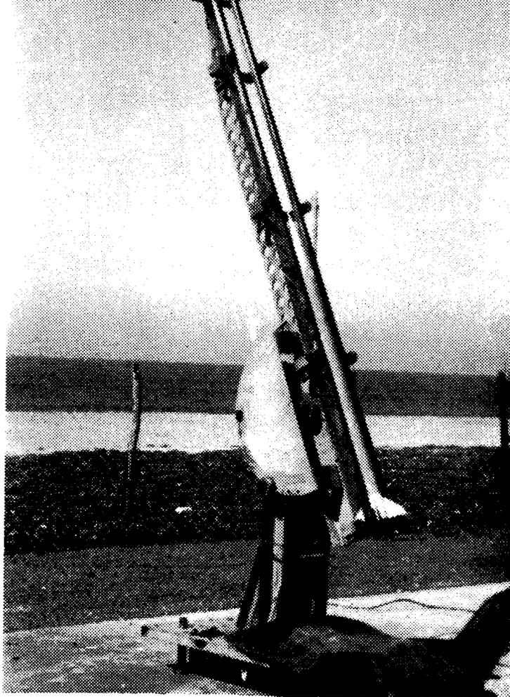
The simple mobile launcher with the Rohini installed.
