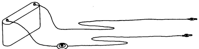
Figure 2. Firing circuit, 1958, similar to that illustrated on Model Missiles, Inc. instruction sheets. The system used a 6V hot-shot battery, a doorbell button, two 10-foot lengths of No. 18 wire, and two Muller No. 85 alligator clips to provide electrical energy for ignition.
