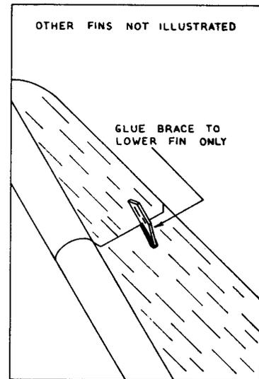
Figure 2. Braces at interstage fin joints.
