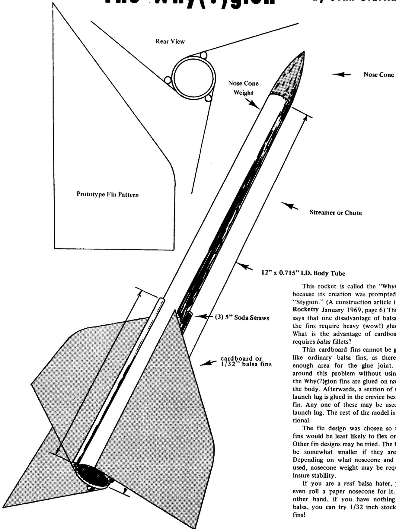
This rocket is called the "Why(?)gion" because its creation was prompted by the "Stygion." (A construction article in *Model Rocketry* January 1969, page 6) This article says that one disadvantage of balsa is that the fins require heavy (wow!) glue fillets. What is the advantage of cardboard if it requires *balsa* fillets?
