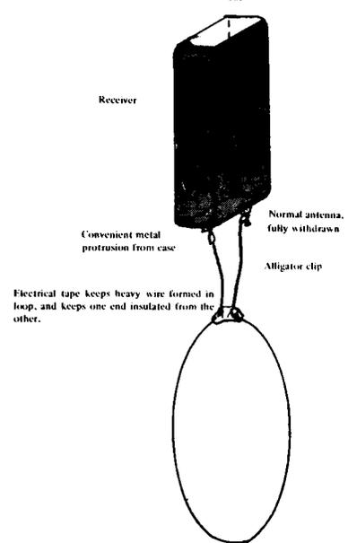
Electrical tape keeps heavy wire formed in loop, and keeps one end insulated from the other.
