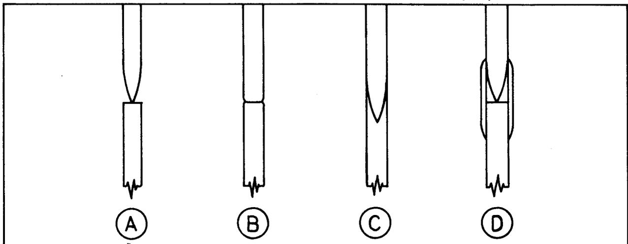
Figure 4. Forms of interstage fin joints. A: sharp trailing edge to flat leading edge, the most common form. B: flat trailing edge to flat leading edge, reduces drag before staging but increases it afterwards. C: sharp trailing edge to form-fitting leading edge, impractical to manufacture. D: sharp trailing edge to cup leading edge, good but involves frontal area penalty.
