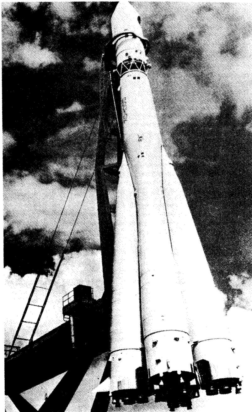
Shown at the U.S.S.R. Exhibition of Economic Achievement in 1967 was the Vostok (A-1) booster, identified as the vehicle which carried Cosmonaut Yuri Gagarin into man's first earth orbit in 1961. Evolved from the original Soviet ICBM, the basic "A" version, without upper stages, orbited the early Sputniks. Configuration shown above has the basic 1½-stage first stage plus first-generation orbital stage.
