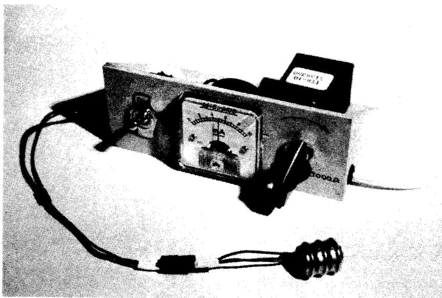
A homemade low-current nicad battery recharger (note the 50 milliamp-hour battery pack in the foreground).
