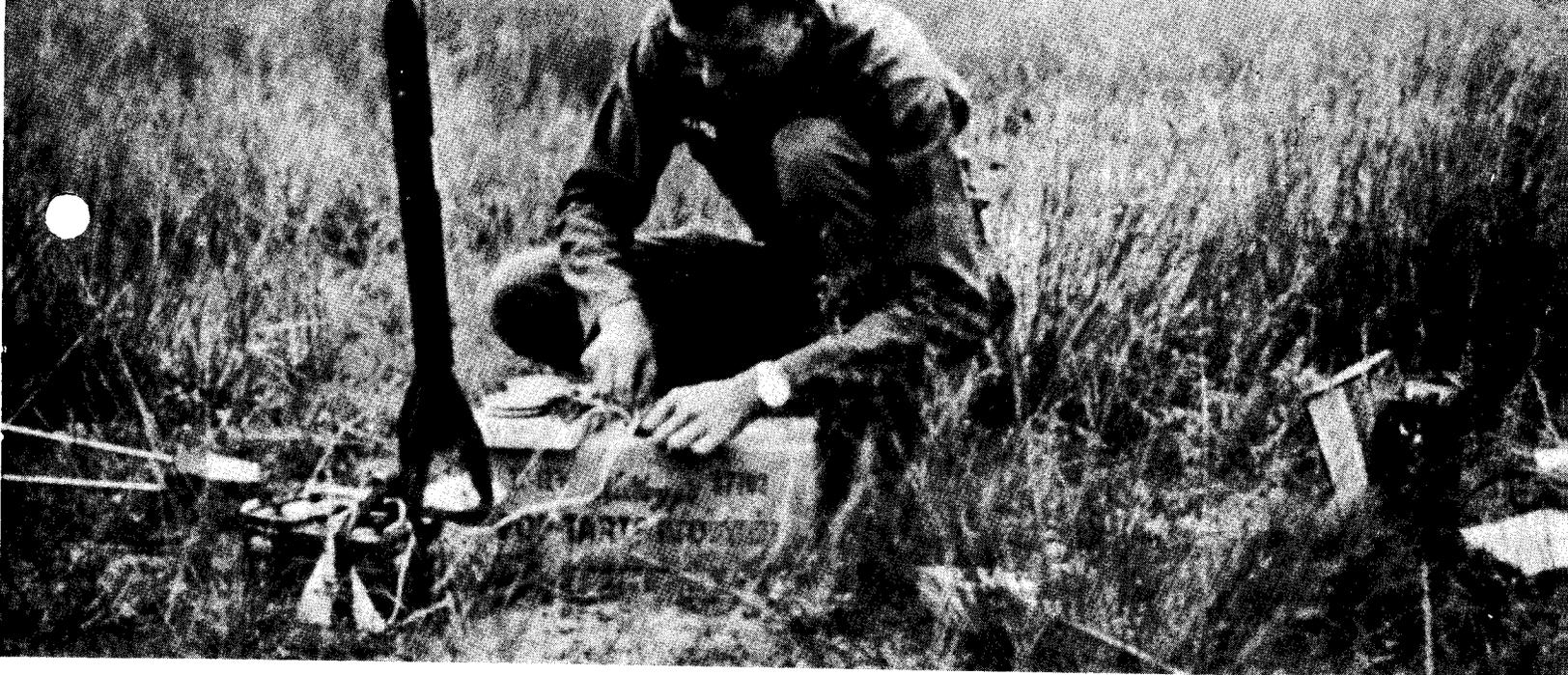
Mims prepares his radio-controlled rocket for a launching from the Saigon Racetrack in South Vietnam. The flight of the ram-air guided rocket was programmed by a tape in the tape recorder at right. The tape sequence was activated at liftoff by a microswitch under the rocket.
